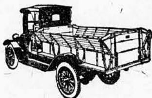
No. 5 Top section folded in and flared—for corn cobs, grain in sacks or other similar loads.
