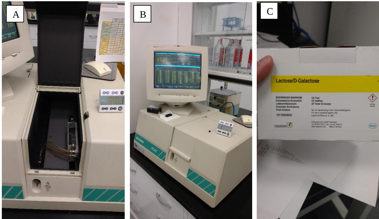
Figure C-1 Equipment and materials used for enzymatic spectrophotometric absorbance reference testing: A) Sample holder and chamber. B) Beckman-Coulter DU- 650 UV-VIS spectrometer. C) Lactose/D-Galactose reagent kit.
