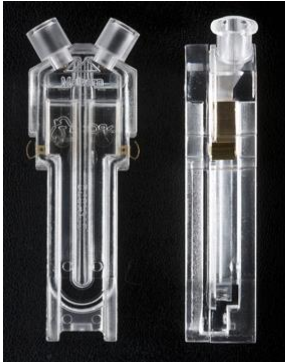
Figure 4-8- Malvern Instruments Zetasizer cuvette front and side view. Gold-plated electrodes pictured allow for the inducing of particle motion with an applied alternating current and voltage power supply. Laser scattering occurs at the bottom.
