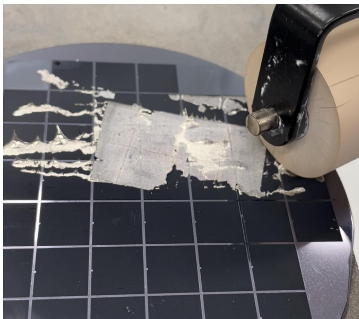
Figure 5-10 - ParyFree coated MSND wafer, with molten lithium being pressed against the trenches by a silicone manual roller.
