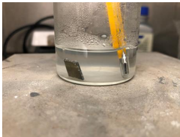
Figure 5-4 - LiF-backfilled MSND upright in a beaker with heated EC:LiF mixture. Diode trenches are exposed to the solution and the temperature drop is measured.
