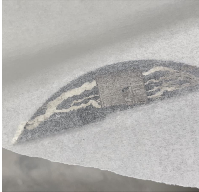
Figure 5-7 - A Parylene-N coated wafer, sandwiched between parchment paper (cellulose), which was pressed with a manual roller above 200 °C on a hot plate. Lithium was successfully melted without violent reactions.
