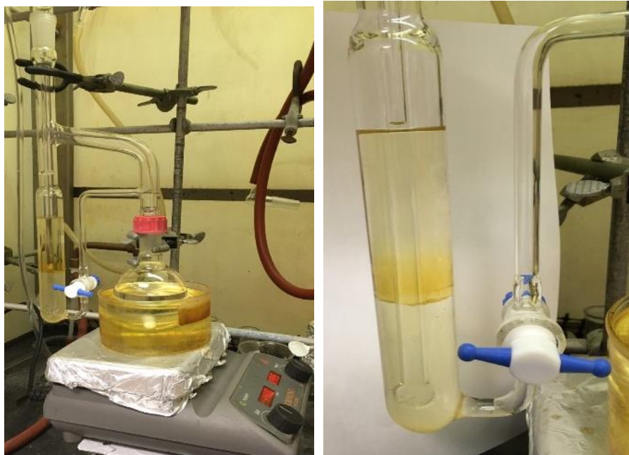
Figure 3.5 The continuous extraction apparatus. Right side- Extraction of pyrazole derivatives from aqueous layer to Ethyl acetate (Top-EtOAc, Bottom Aq).
