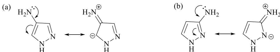
Scheme 2.10 The Lewis resonance structures of 4-aminopyrazole and 3-aminopyrazole to show the delocalization of the nitrogen's lone pair to the pyrazole ring.
