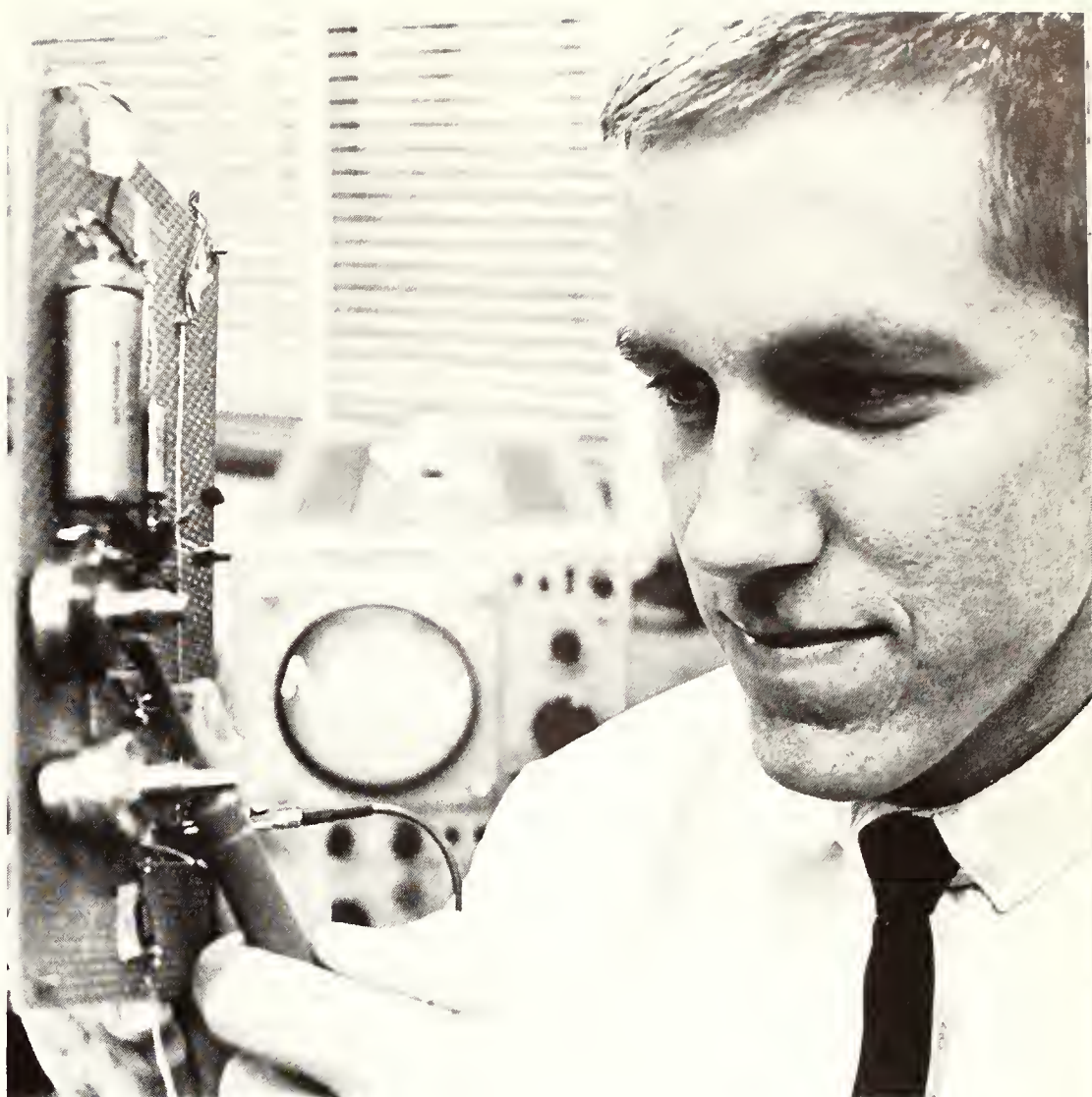
Electrical engineering student Jack Crumrine tests a resistor with a triangular wave generator circuit.
