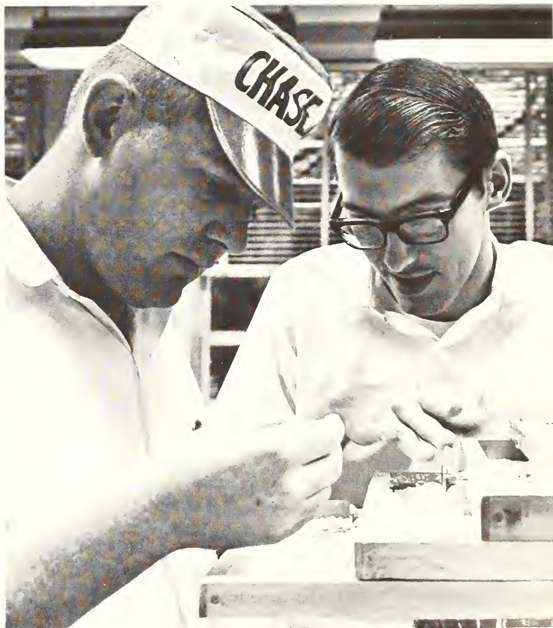
While sifting corn meal, milling students analyze it for the protein content per size of particle.
