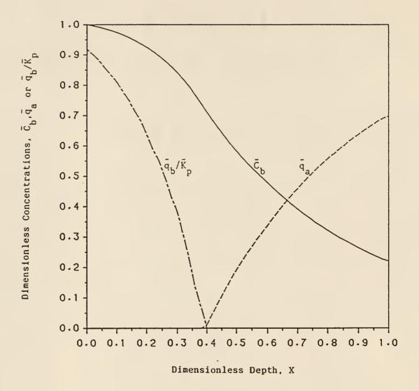
Figure 3.7. Concentration profiles of base in the solution, acid in the soil, and base in the soil at  $\theta$ =10: Pe=100, St =2,  $R_0$ =0.05 and  $\bar{K}_p$ =4.
