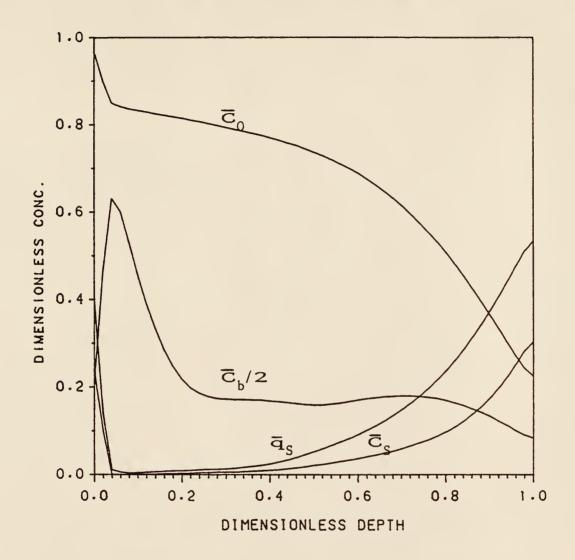
Figure 4.11. Concentration profiles for the recycle operation at  $\theta{=}8\colon$  Da'=0.2, R  $_S{=}20$  and W=8.
