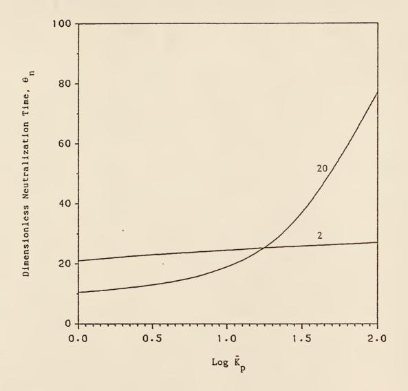
Figure 3.8. Effect of  $\bar{K}_p$  on the dimensionless neutralization time with St as the parameter: Pe=100 and R \_0=0.05.
