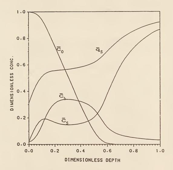
Figure 4.3. Concentration profiles for the once-through operation at  $\theta\text{=}3\colon$  Da'=0.5, R  $_S\text{=}20$  and W=12.5.
