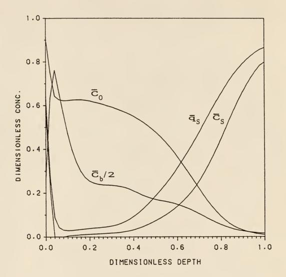
Figure 4.10. Concentration profiles for the recycle operation at  $\Theta\text{=}6$  : Da'=0.2, R  $_{S}\text{=}20$  and W=8.
