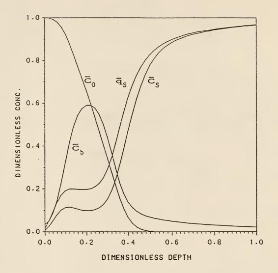
Figure 4.4. Concentration profiles for the once-through operation at  $\theta\text{=}3\colon$  Da'=0.1, R  $_S$  =20 and W=12.5.
