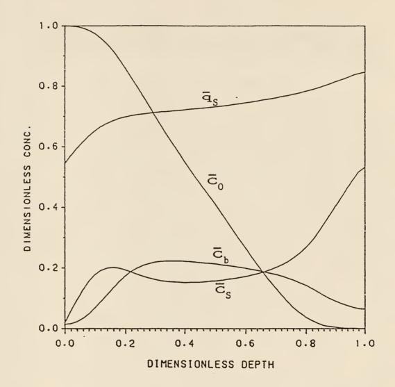
Figure 4.2. Concentration profiles for the once-through operation at  $\theta$ =3: Da'=1, R =20 and W=12.5.
