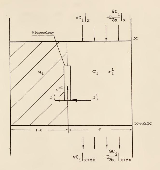
Figure 4.1. Schematic diagram of transport and biodegradation in a controlled volume.
