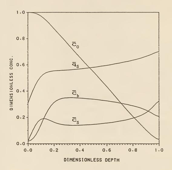
Figure 4.6. Concentration profiles for the once-through operation at  $\theta\text{=}3\colon$  Da'=0.5, R  $_{S}\text{=}20$  and W=6.
