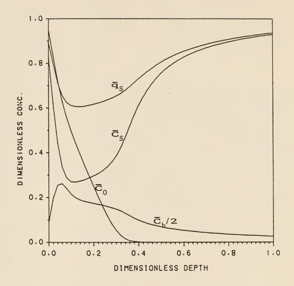
Figure 4.8. Concentration profiles for the recycle operation at  $\theta\text{=}2\text{:}$  Da'=0.2, R =20 and W=8.
