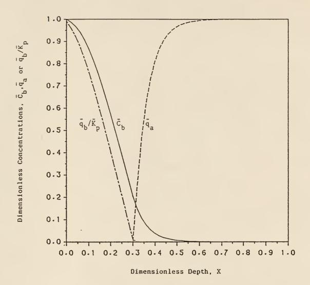
Figure 3.3. Concentration profiles of base in the solution, acid in the soil, and base in the soil at  $\theta$ =10: Pe=100, St =20,  $R_0=0.05 \text{ and } \vec{K}_p=40.$
