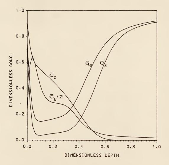
Figure 4.9. Concentration profiles for the recycle operation at  $\theta\text{=}4:$  Da'=0.2, R  $_{S}\text{=}20$  and W=8.
