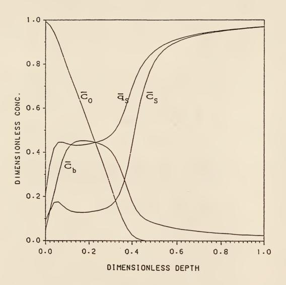
Figure 4.5. Concentration profiles for the once-through operation at  $\theta\text{=}3\colon$  Da'=0.1, R  $_S$  =60 and W=12.5.
