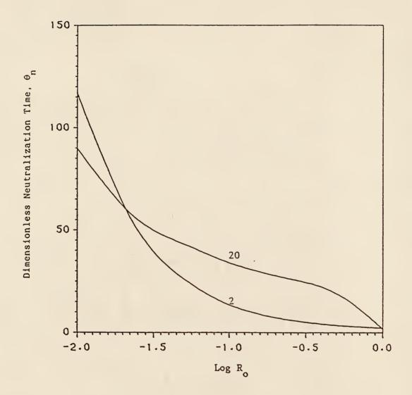
Figure 3.6. Effect of R  $_0$  on the dimensionless neutralization time with St  $_m$  as the parameter: Pe=100 and  $\overline{\rm K}_p$ =40.
