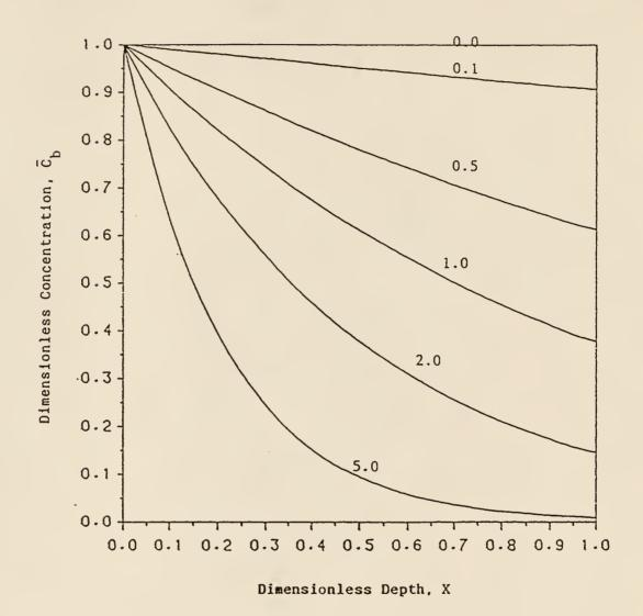
Figure 3.1. Effect of St  $_{m}$  on the concentration distribution of base in solution at  $\theta$ =10 with St  $_{m}$  as the parameter: Pe=100,  $R_{o}$ =0.0125 and  $\bar{K}_{p}$ =40.
