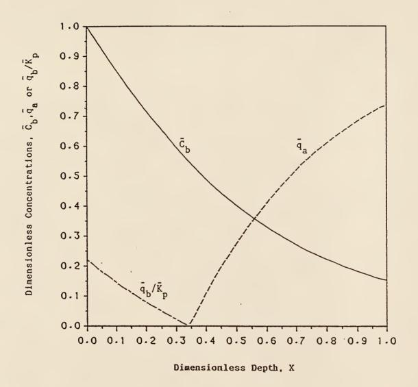
Figure 3.2. Concentration profiles of base in the solution, acid in the soil, and base in the soil at  $\theta$ =10: Pe=100, St<sub>m</sub>=2,  $R_0$ =0.05 and  $\bar{K}_p$ =40.
