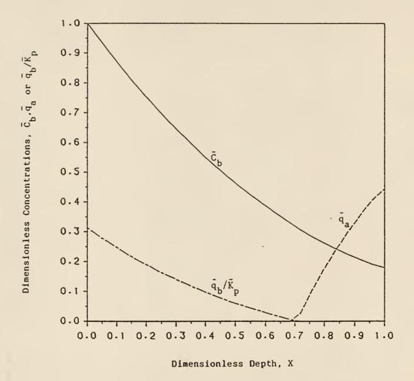
Figure 3.5. Concentration profiles of base in the solution, acid in the soil, and base in the soil at  $\theta$ =10: Pe=100, St<sub>m</sub>=2,  $R_0=0.1 \text{ and } \bar{K}_p=40.$
