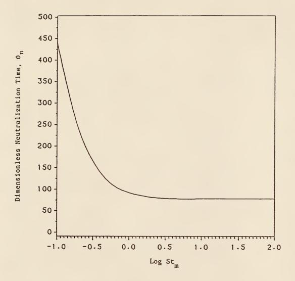
Figure 3.4. Effect of St  $_m$  on the dimensionless neutralization time:  $Pe=100,\ R_0=0,0125\ and\ \bar{K}_p=40\,.$
