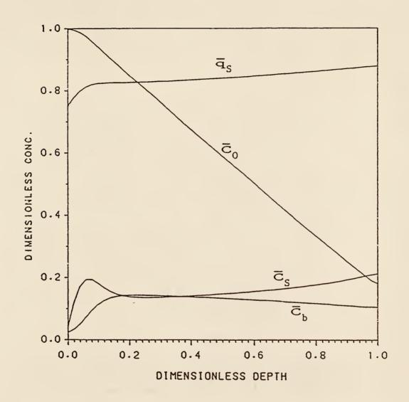
Figure 4.7. Concentration profiles for the once-through operation at  $\theta\text{=}3\colon$  Da'=0.5, R  $_S\text{=}80$  and W=12.5.
