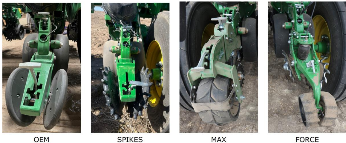
Figure 4.3. Rear view of the closing wheel designs (CWD) tested in the experiment. OEM: round rubber closing wheel (Deere & Company, Moline, IL); SPIKES: Twisted Spikes wheels (Yetter Farm Equipment, Colchester, IL); MAX: Furrow Max™ closing system (Yetter Farm Equipment, Colchester, IL); FORCE: FurrowForce® closing system (Precision Planting, Tremont, IL).
