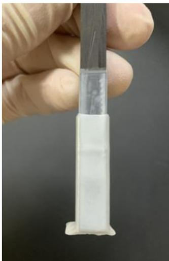
**Figure 5.2.** Preparation of the parafilm holder for coating process.
