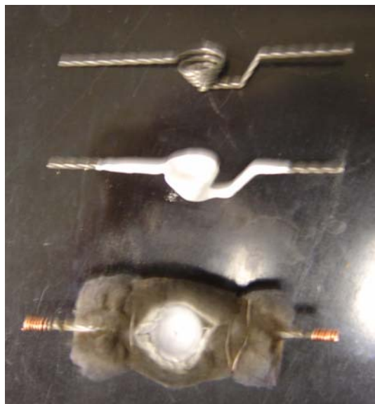
Figure 3 - Preparation of crucibles for metal evaporation. A wire basket is purchased for use, coated with aluminum oxide cement, contact points are wrapped in copper wire, and finally insulation with alumina mat is secured around the outside of the crucible.
