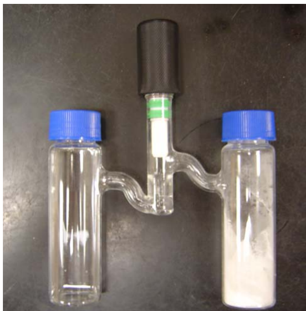
Figure 58 - Apparatus used to control the evaporation of solvent from a nanoparticle colloid to induce slow precipitation of the colloid.
