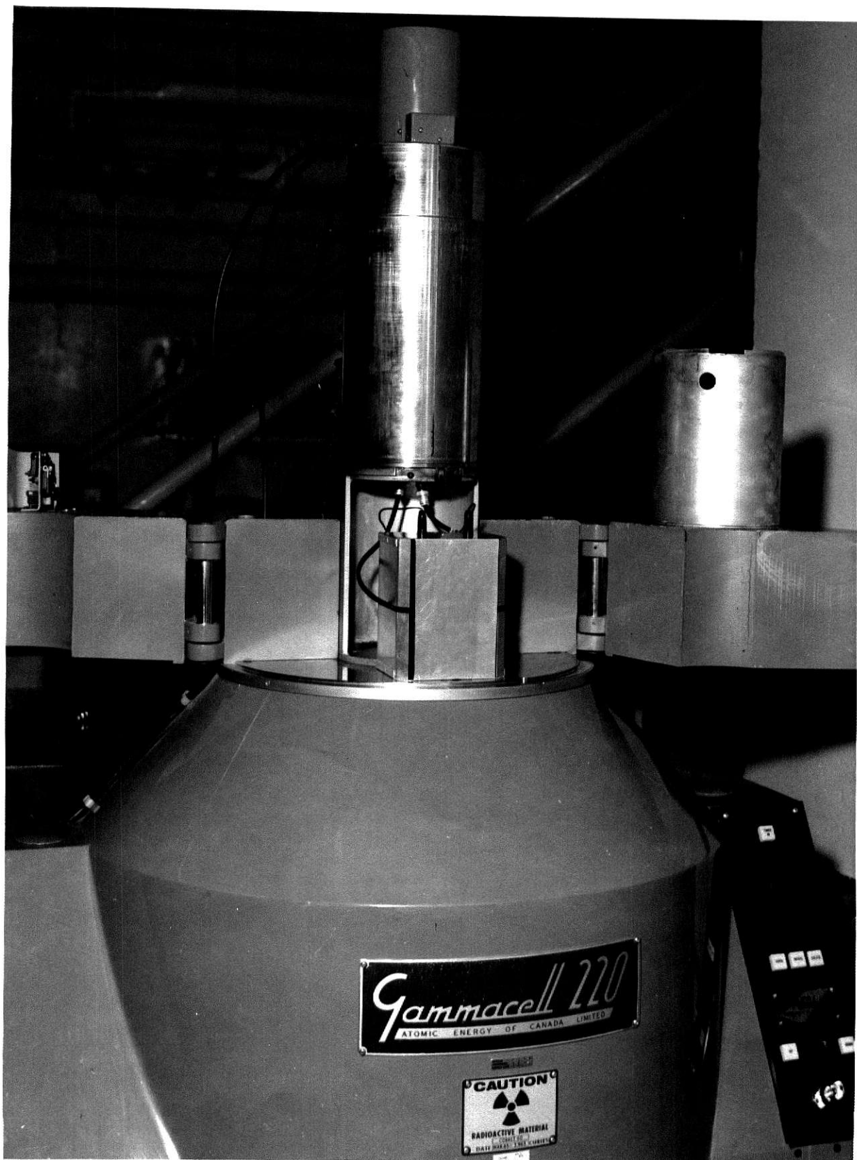
Fig. I-5. Electrical hookup and positioning of testing box.
