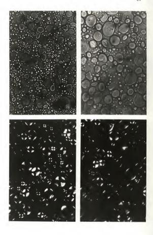
Figure 17. Photomicrographs both bright field and polarized light of the same field. Doughs were heated to 68°C in the electric resistance oven. Doughs (15 g) containing shortening (left) and no shortening (right) were dispersed in water (100 ml).
