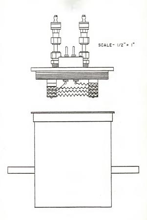
insulate and feed the electrical wire to the outside. The external male plug, mounted in "lavelite", is fixed to the top of the lip and is a permanent connection point. The female electrical connections are also mounted in "lavelite" and asbestos wire is used to bring current to the baking container.
