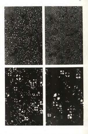
Figure 16. Photomicrographs both bright field and polarized light of the same field. Doughs were heated to  $64^{\circ}\text{C}$  in the electric resistance oven. Dough (15 g) containing shortening (left) and no shortening (right) was dispersed in water (100 ml).
