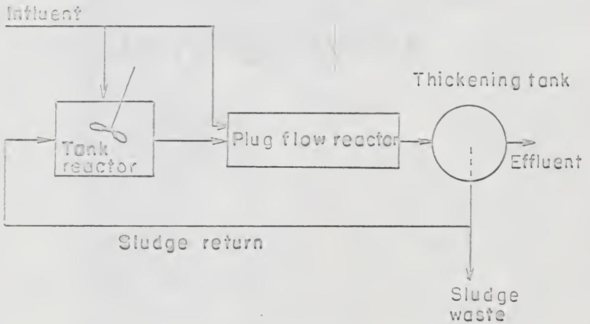
Fig. 23. Schematic diagram of composite system.
