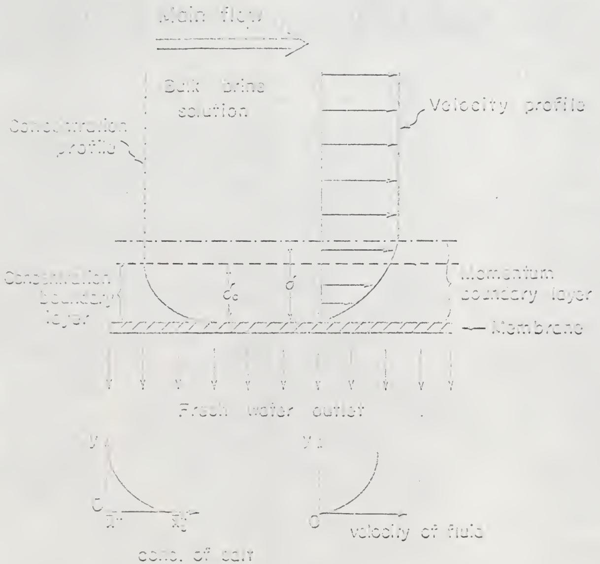
Fig. 1. Velocity and salt concentration gradients in boundary layer adjacent to a membrane.
