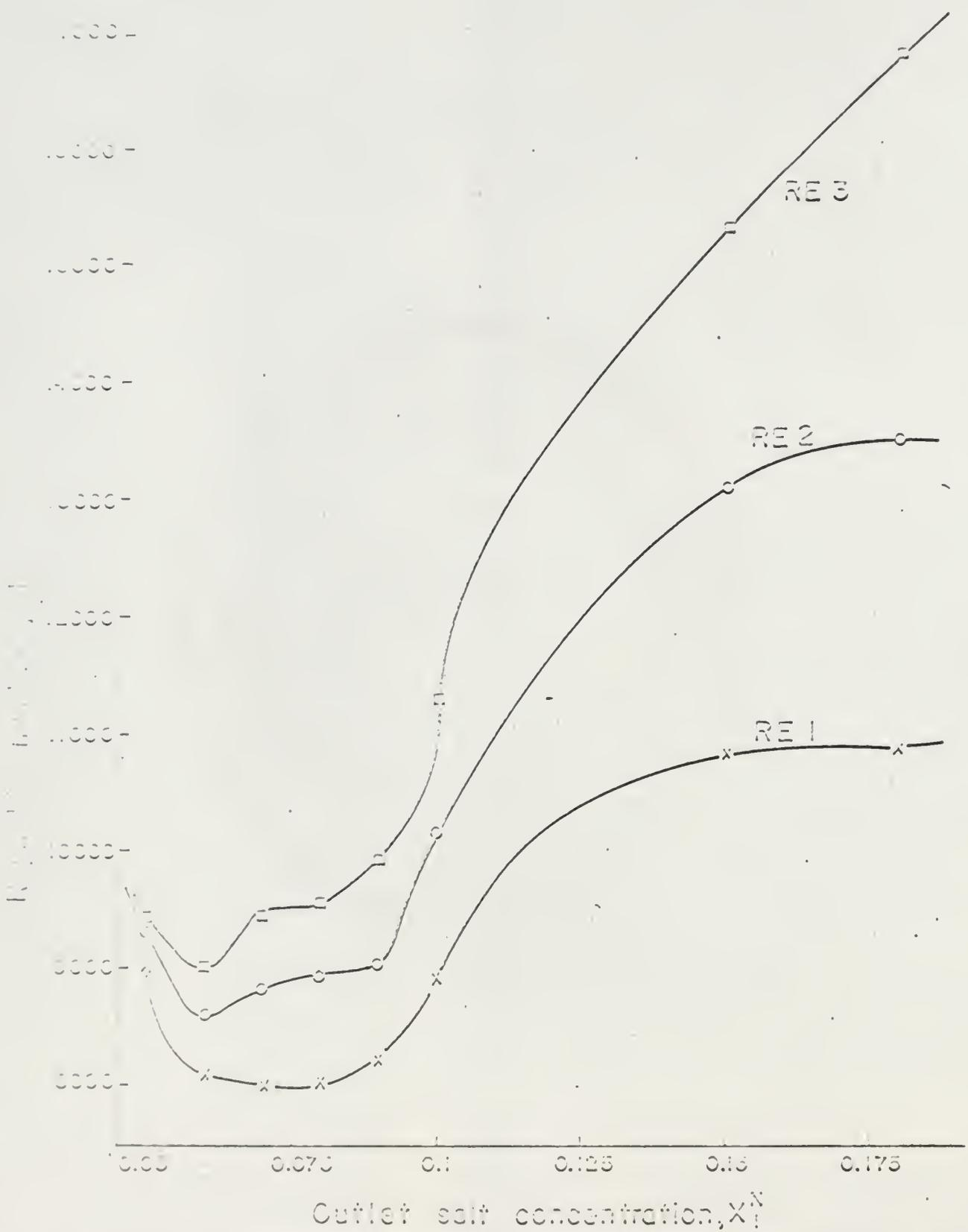
Fig. 5 Optimal Reynolds number vs exit salt concentration for a three stage system with a flow work exchanger.
