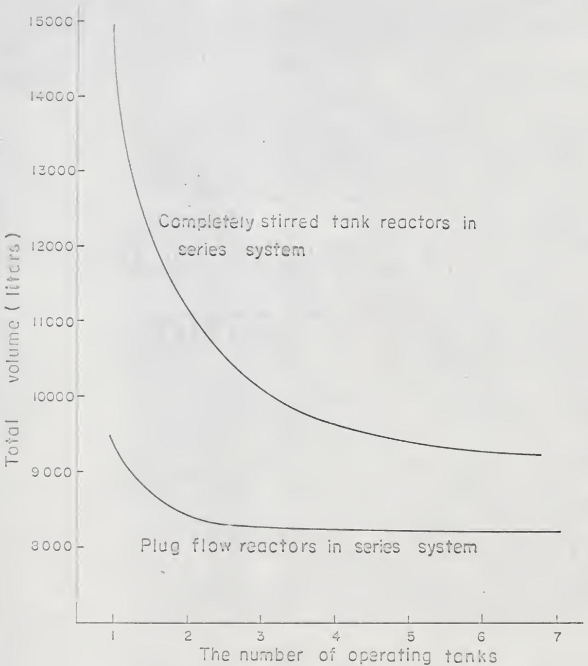
Fig.19. Comparison of completely stirred tank reactor systems and plug flow reactor systems for step aeration process.
