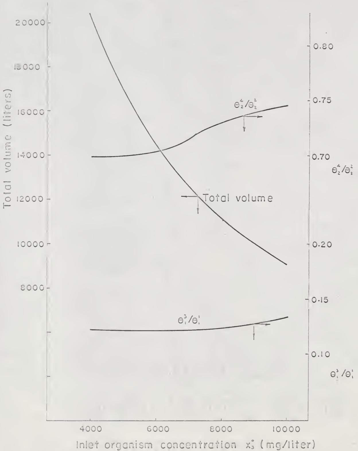
Fig. 15. Optimal total volume, feed distribution ratio, and volume distribution ratio as functions of the inlet organism concentration for the two tank step aeration system.
