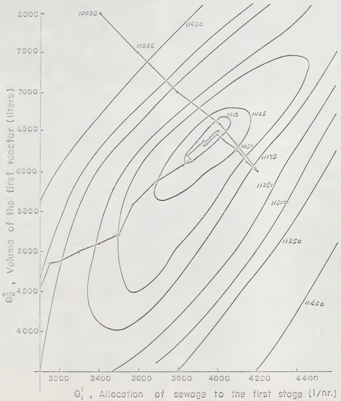
Fig. 12. Surface contours for the system and the searching locuses.
