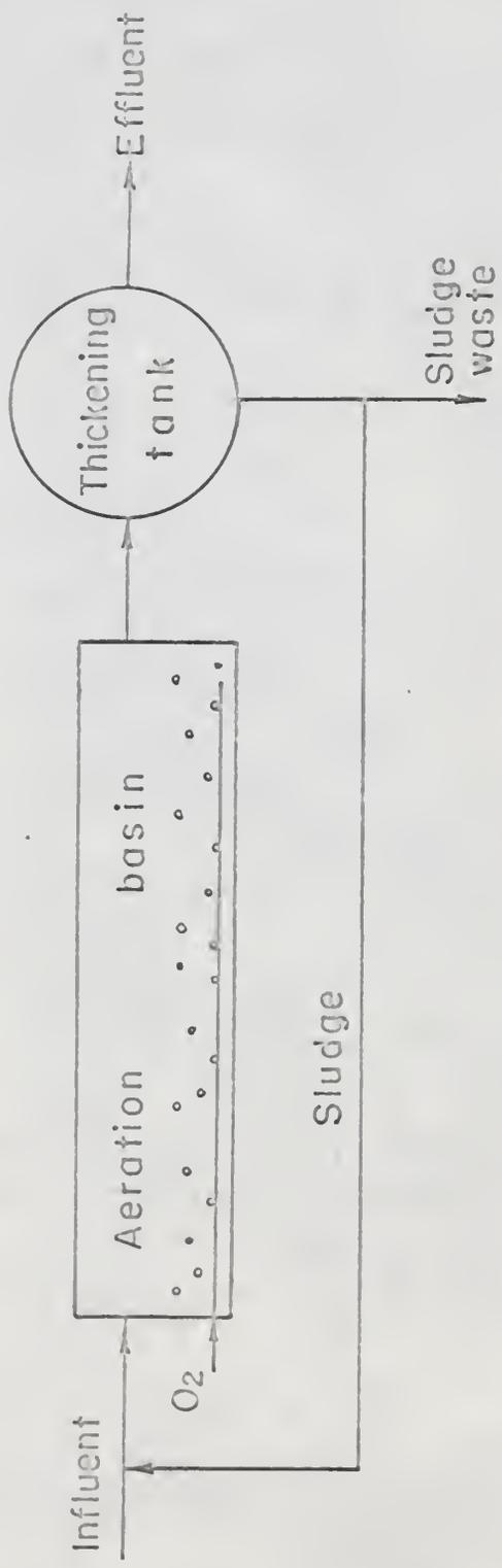
Fig. 2 . Flow diagram of conventional activated sludge process.
