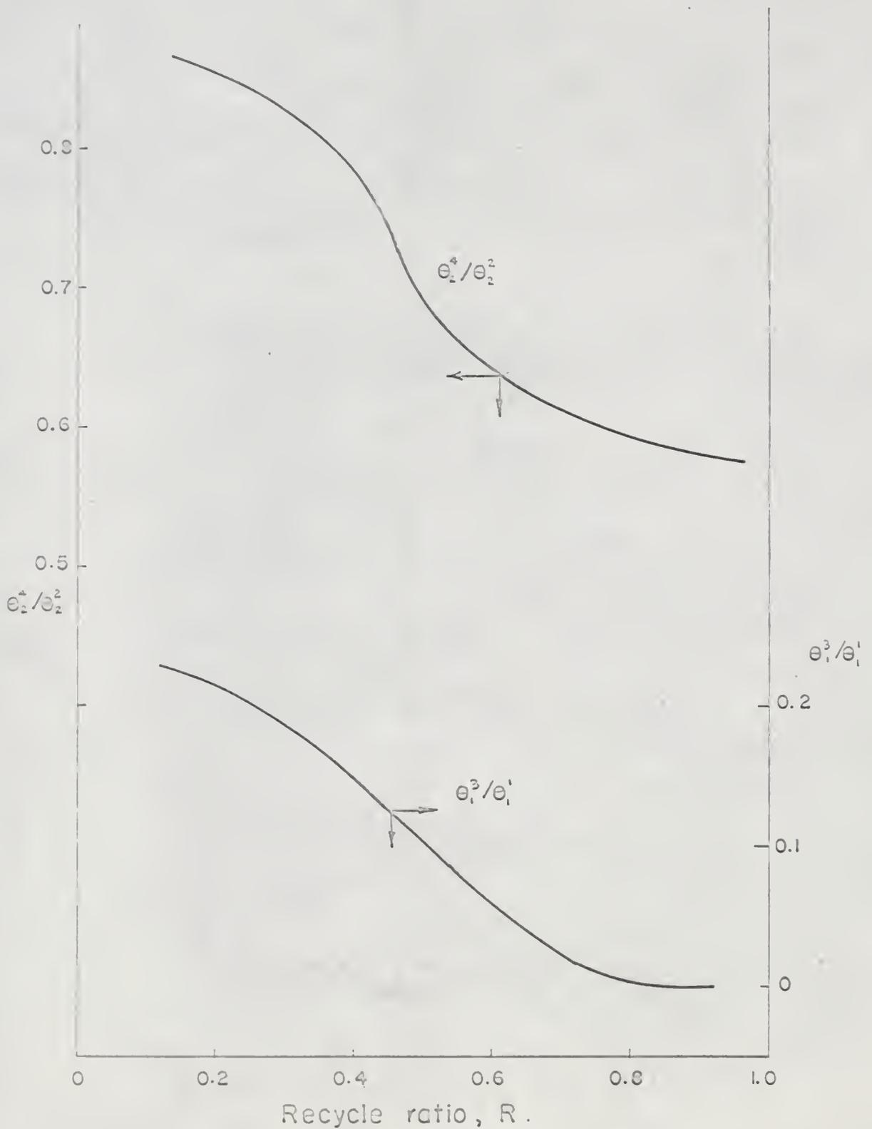
Fig. 13. Optimal feed distribution ratio and volume distribution ratio as function of recycle ratio for the two tank step aeration system.
