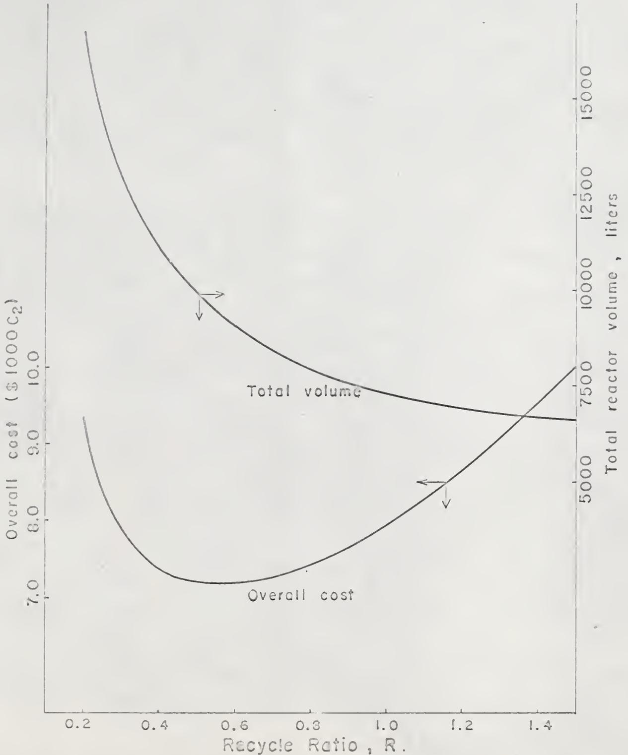
Fig.17. Overall cost and total volume v.s. recycle ratio for the two completely stirred tank step aeration system.
