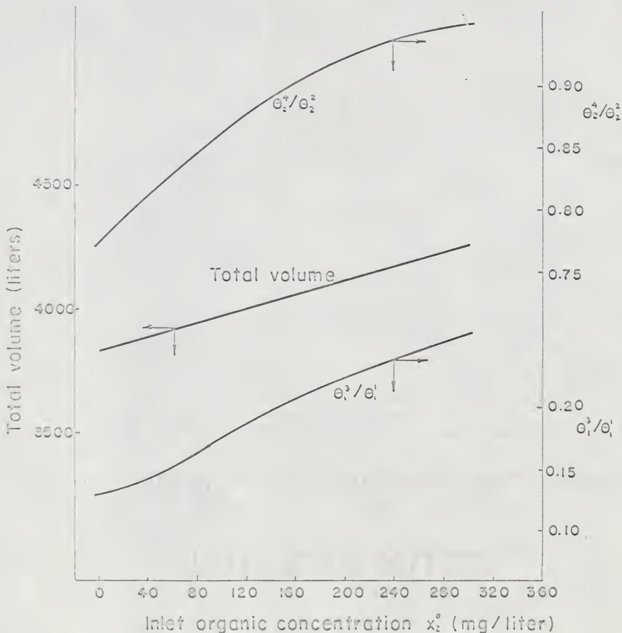
Fig. 16. Optimal total volume, feed distribution, and volume distribution ratio as functions of inlet organic for the two tank aeration system.
