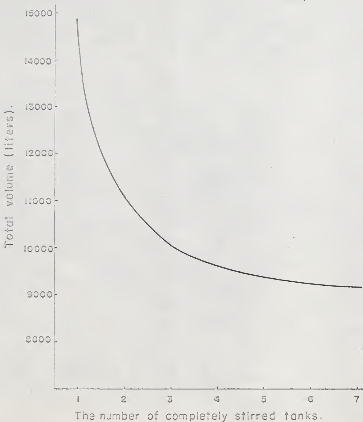
Fig. 14. Optimal total reactor volume v.s. the number of operating tanks for completely stirred tanks connected in series.
