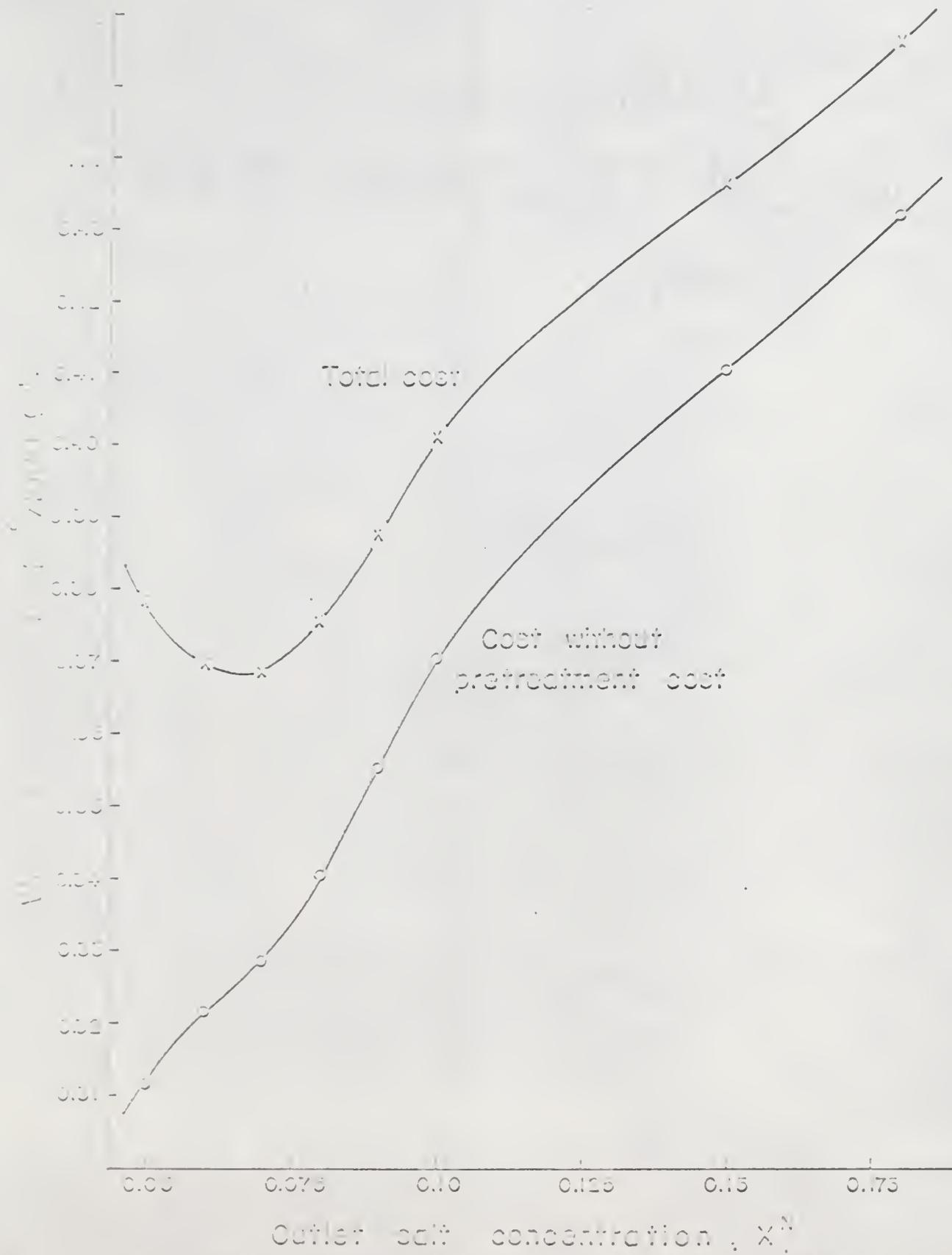
General water production cost vs salt concentration for a three stage system with a flow work
