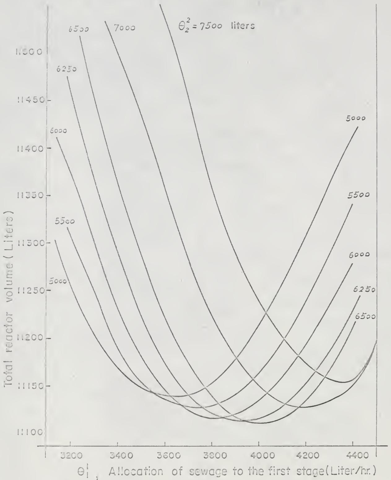
Fig. 11. Overall accumulated volume vs. allocation of sewage to the first reactor with the volume of the first reactor as parameter.
