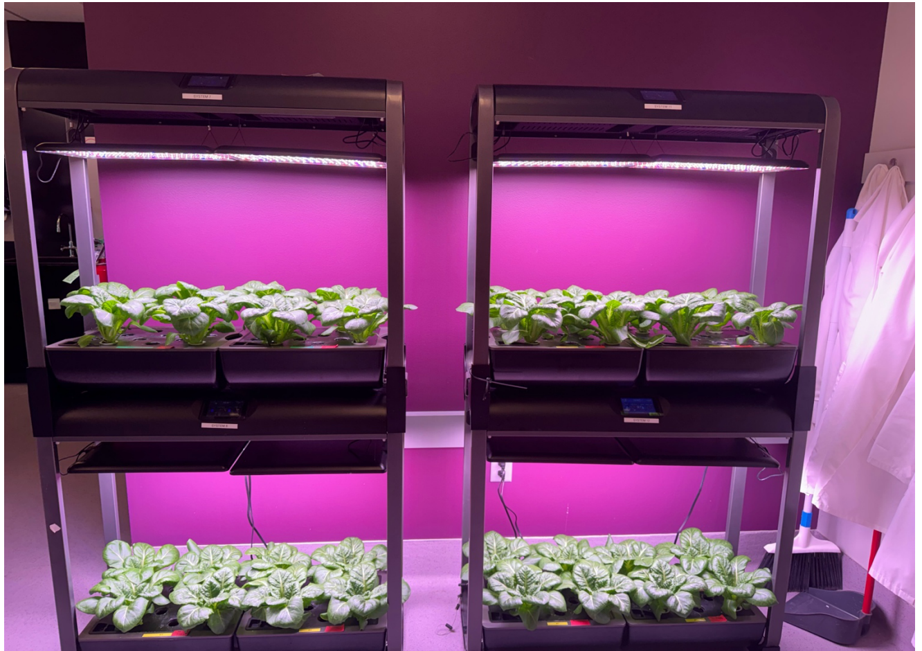
Figure 2. Picture of Deep-water culture of hydroponic system used in our experiment.
