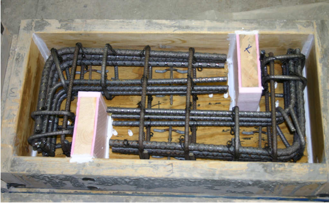
Figure 7.5: Monolithic Specimen Prior to Casting
