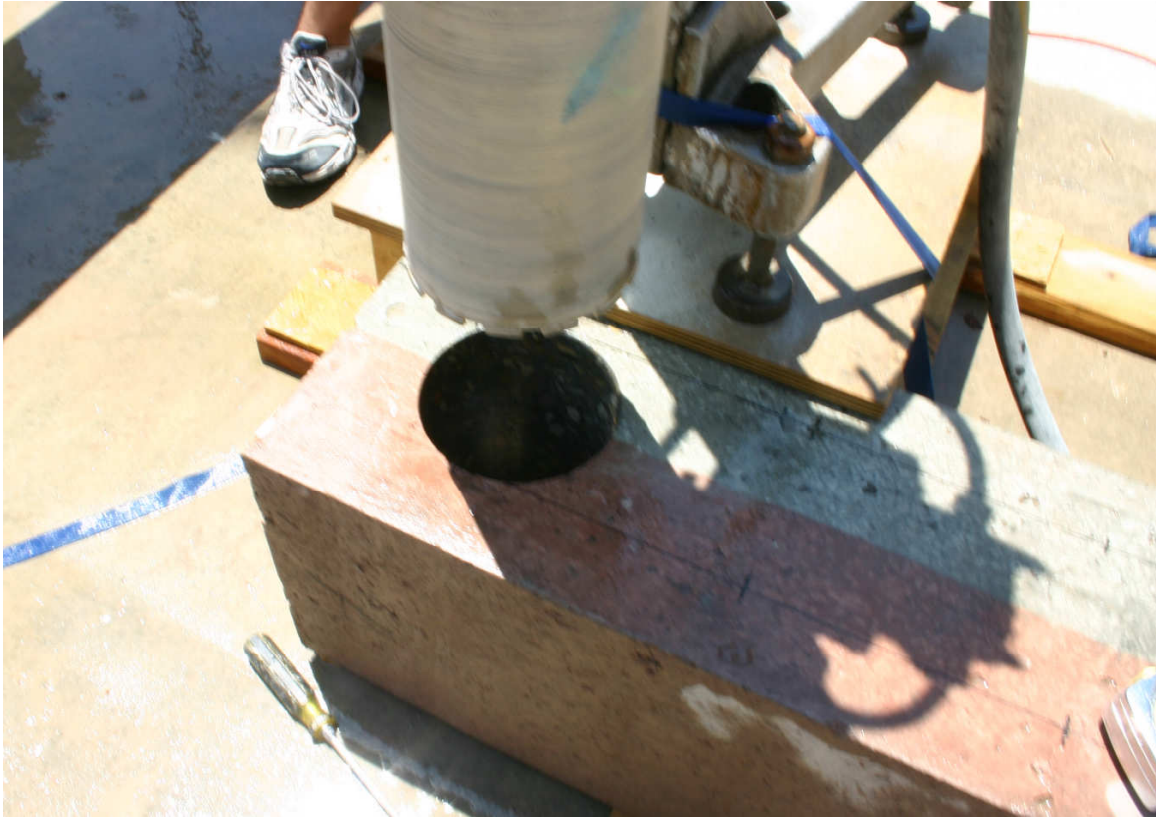
Figure 6.5: Coring of a Small Core Block
