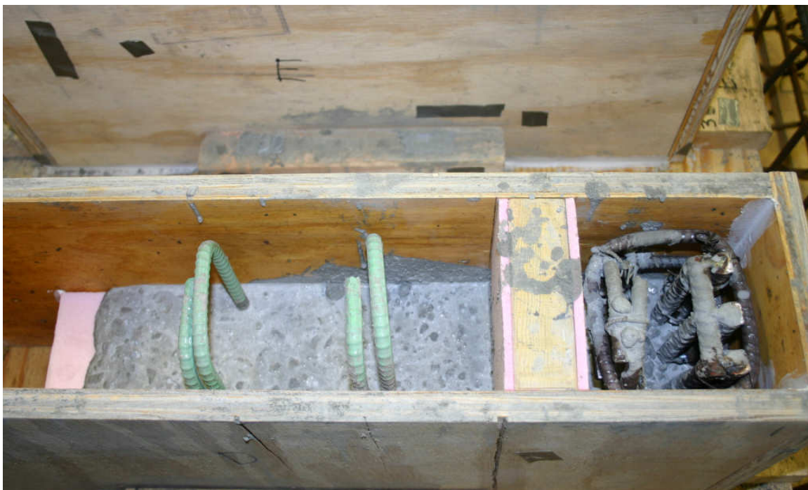
Figure 7.7: Bottom Half of Cold-Joint Specimen
