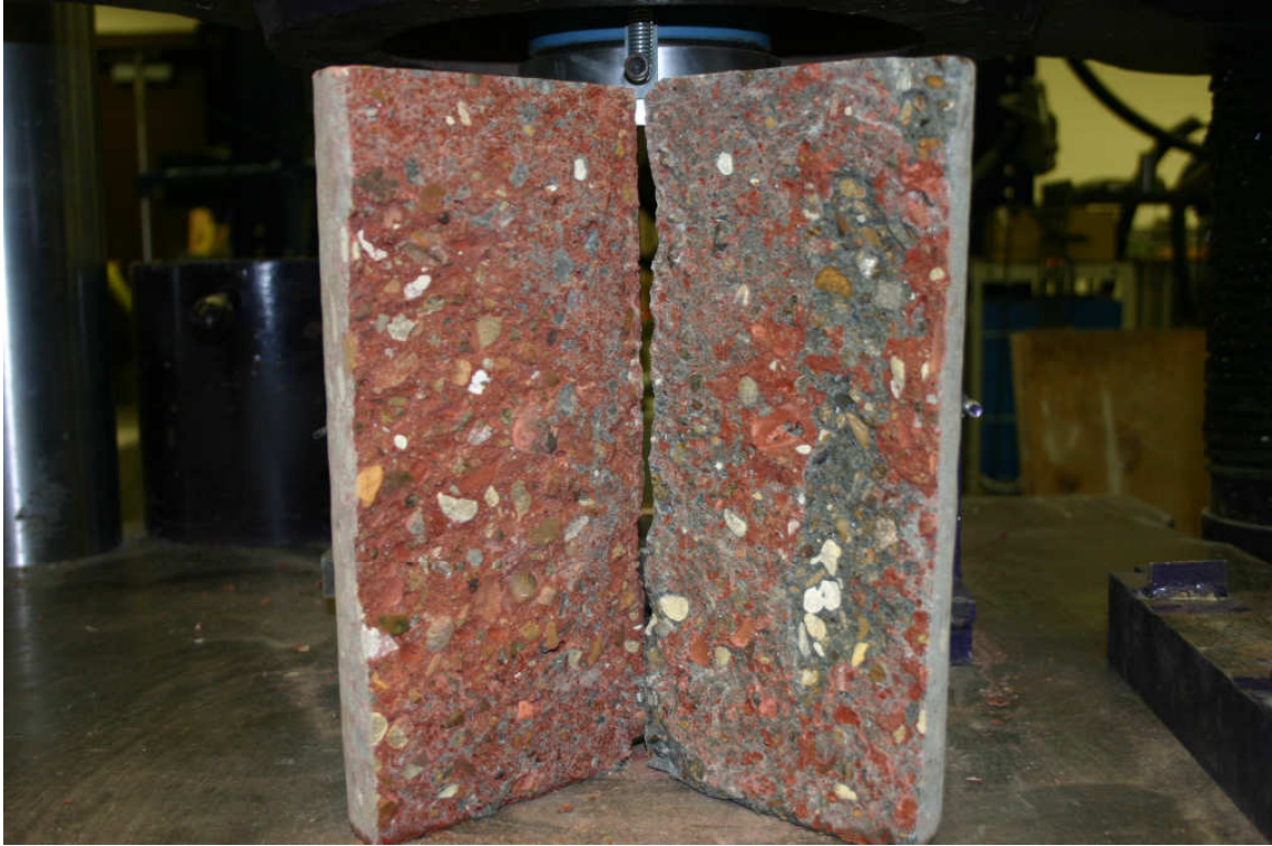
Figure 6.6: Core after Split-Tensile Test
