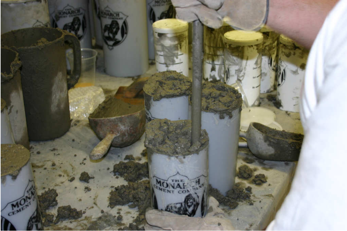
Figure 4.11: Making Concrete Cylinders
