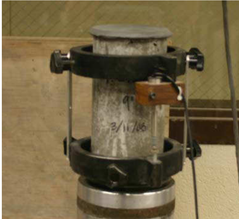
Figure 4.14: Cylinder Mounted with Compressometer
