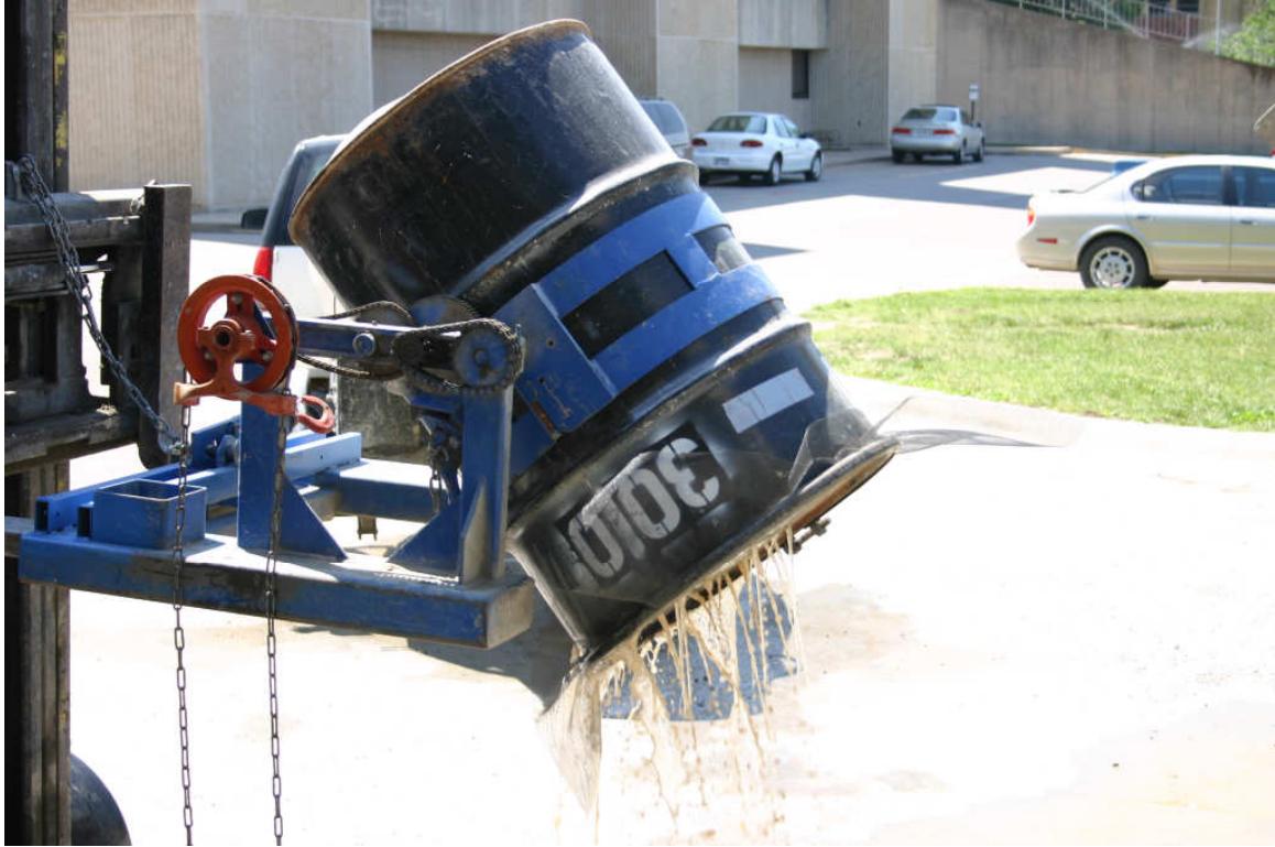
Figure 4.4: Water Being Drained for Large Concrete Batch
