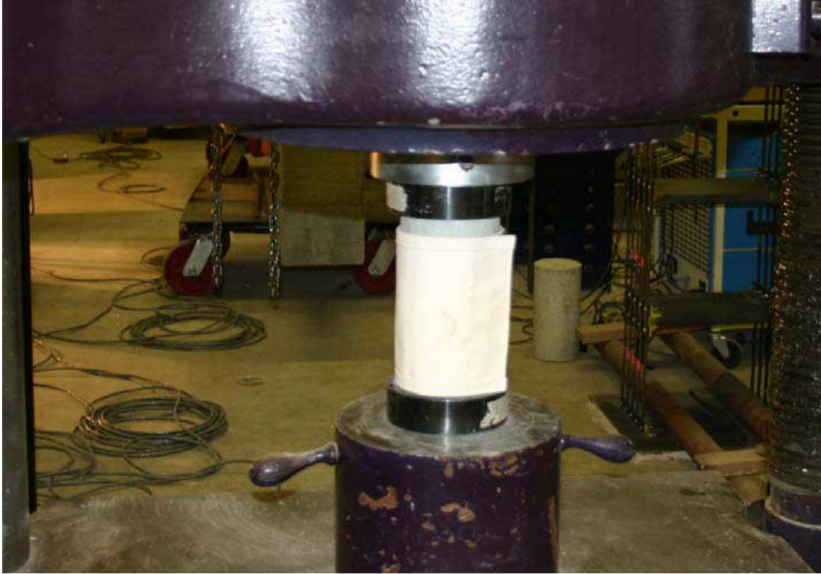
Figure 4.12: Compressive Strength Test
