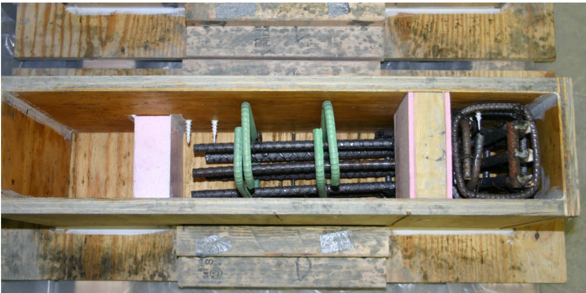
Figure 7.6: Cold-Joint Specimen Prior to Casting
