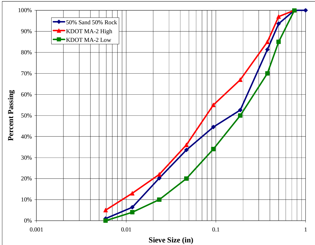
Figure 3.3: Gradation Curve of Mixed Aggregate
