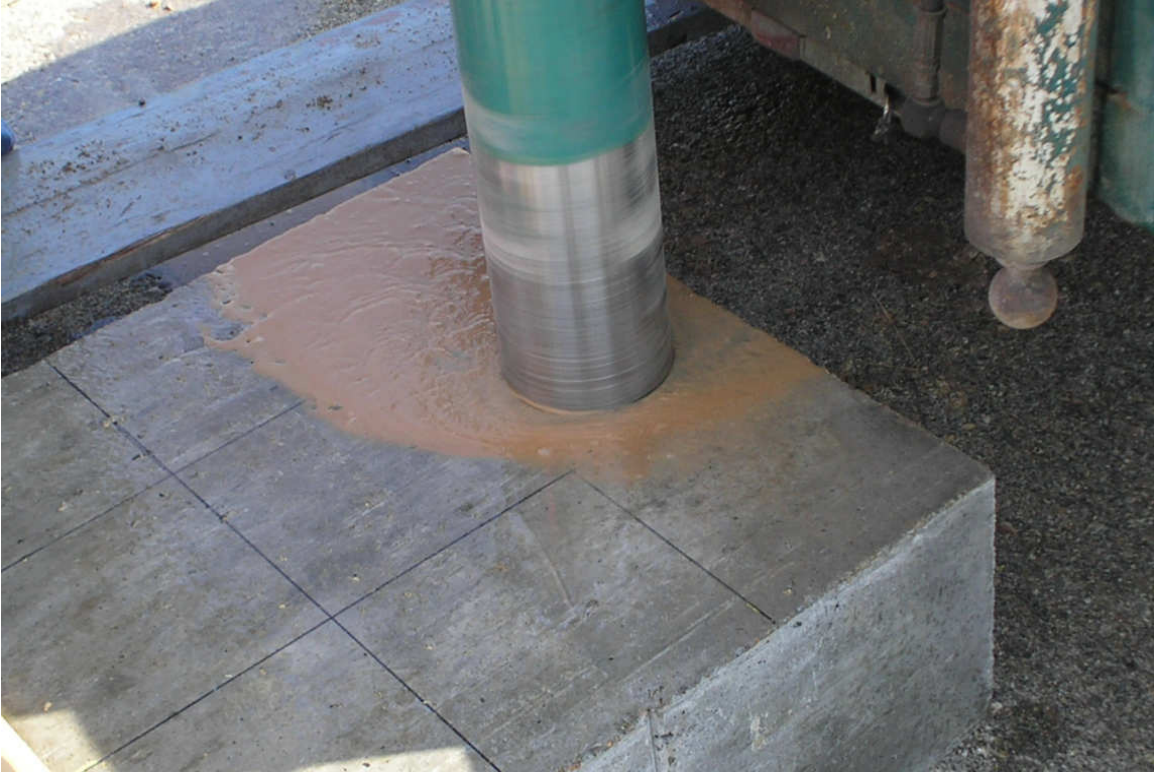
Figure 6.2: Coring of a Large Core Block
