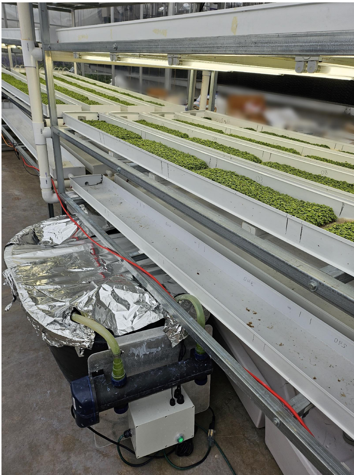
Figure 4.2. Treatment system containing a TiO 2 tank and a UV lamp chamber.
