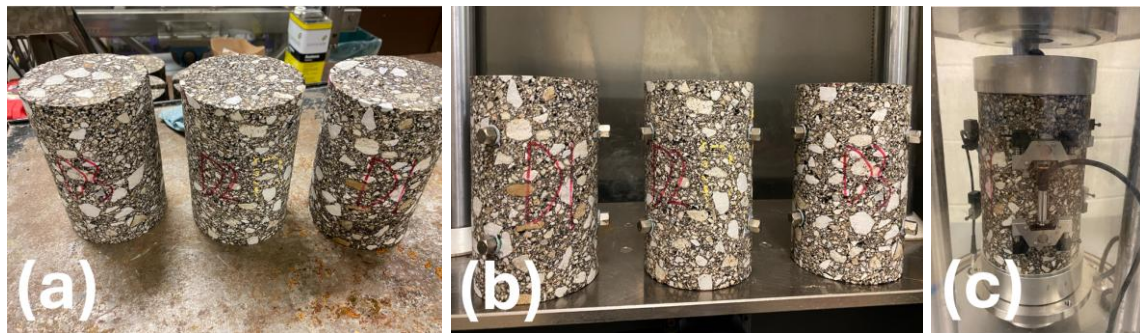
Figure 6.5 Dynamic Modulus of HMA Mixtures
