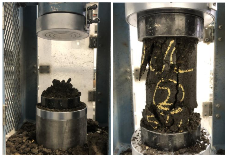
(a) FDR Specimen (b) SFDR Specimen Figure 2.3 Comparison of UCS Test Specimens
