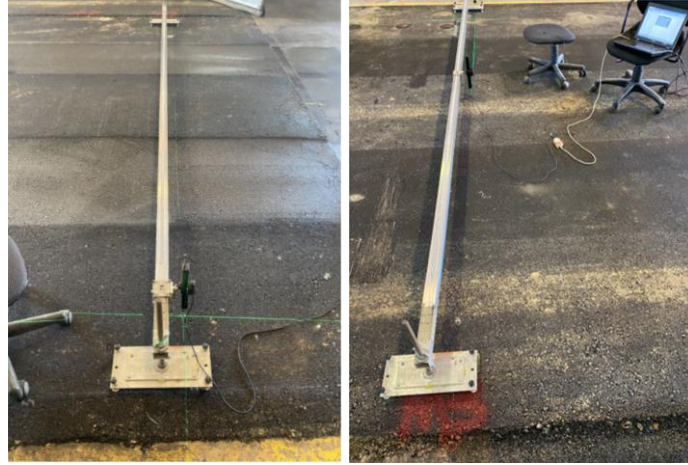
Figure 5.25 Transverse Profile Measurement
