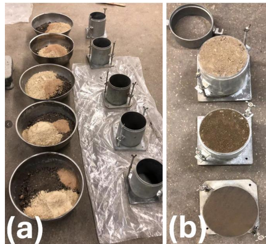
Figure 3.5 Proctor Test for SFDR Mixture: (a) SFDR Material Preparation; (b) SFDR Material Compaction
