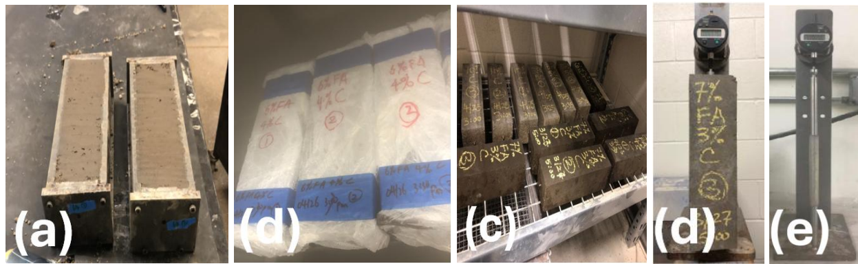
Figure 3.8 Linear-Shrinkage Test: (a) Specimen Preparation; (b) Specimen Curing; (c) Drying; (d) Measurement Device; (e) Length-Reference Comparator
