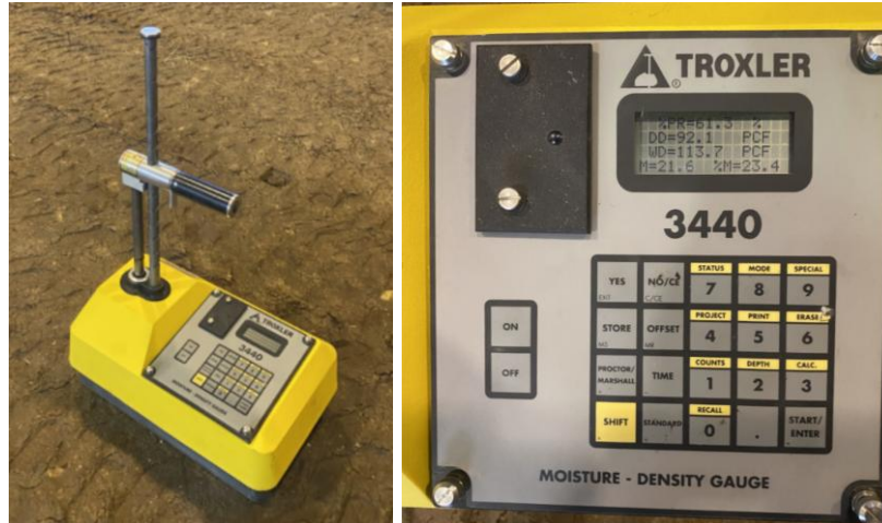
Figure 5.7 Nuclear Gauge Testing
