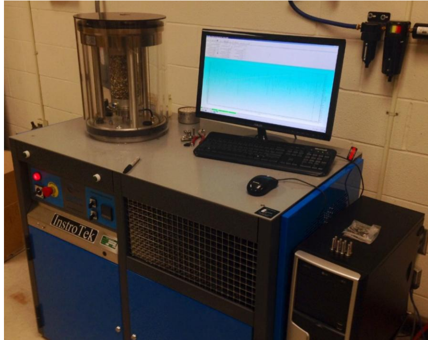
Figure 7.4 Creep Test Setup (Saghebfar, 2014)
