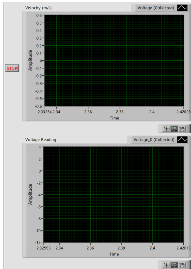
Figure B.2. Front panel of the drop test VI used to display the real time voltage across a resistive load and magnet velocity.
