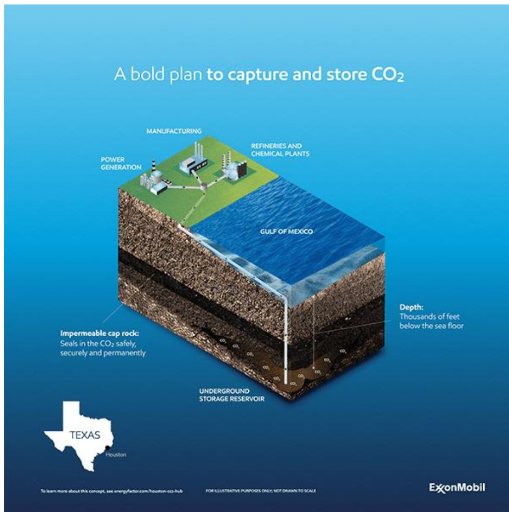
Figure 5. Illustration of proposed method of CO 2 capture in the Gulf of Mexico [15]
