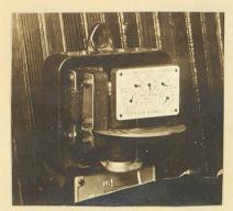
shunt coil is in the back and left side of case; its flux is carried through the laminated core to the disc where it passes through causing the eddy currents which react with the series coils which are above and below the disc. There is an
