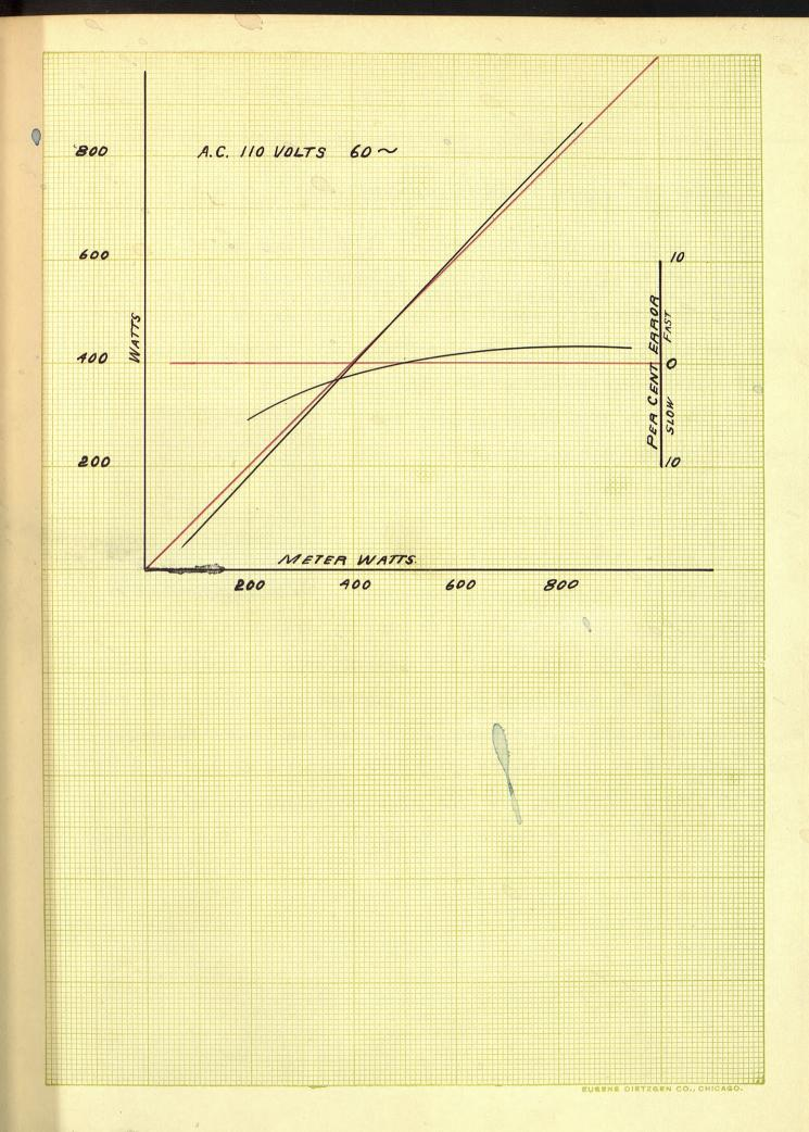
Test on Sangamo Meter No. 15061, 5 Ampers, 110 Volts.
