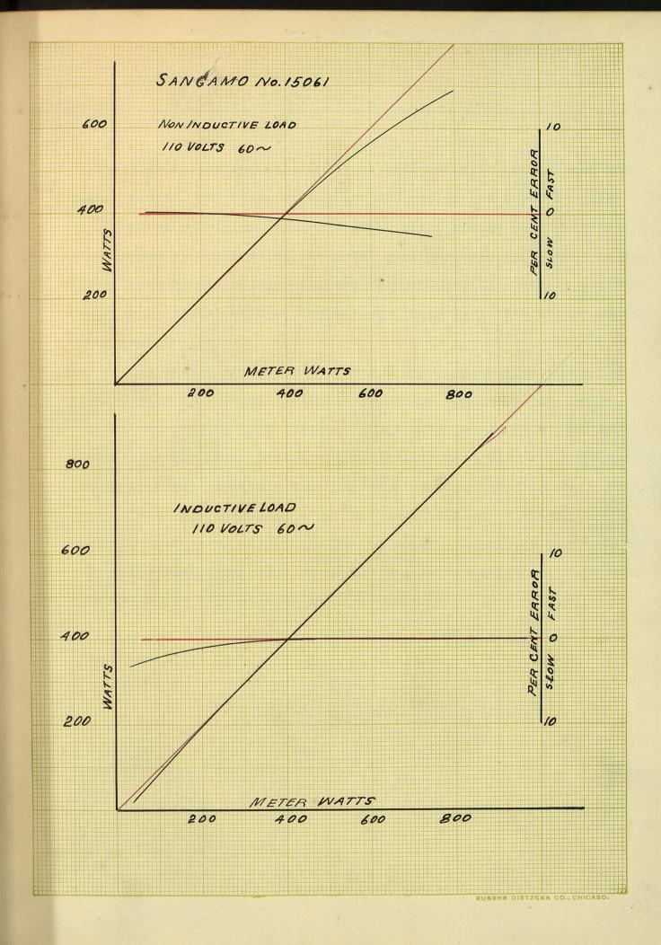
By consulting the curves of this meter it can be seen that under normal conditions of voltage and cycles the meter is quite accurate on non-inductive loads until considerable over full load is reached at which point the meter runs more slowly. With inductive loads normal voltage and cycles the error lies almost entirely with small laads while at large loads there is little error even on over load.
