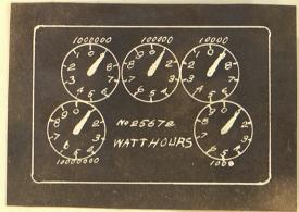
The reading in this case is 09,091,000, instead of 19,191,000, as apparent at first glance.
