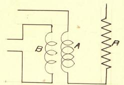
is the movable coil. Coil B. is the stationary coil thru which the current flows. Then the torque is due to the fields of both coils which at any instant is equal to the current at that instant times the voltage at the same instant, which is the
