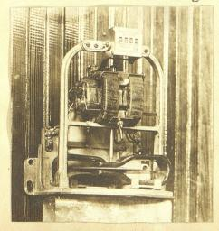
coil is a shunt coil in series with the armature. The damping disc is of copper and the magnets are located far enough away from the coils so that the field of the coils will not demagnetize the magnets. The bearing is a jewel on which a hardened steel point runs. A high resistance
