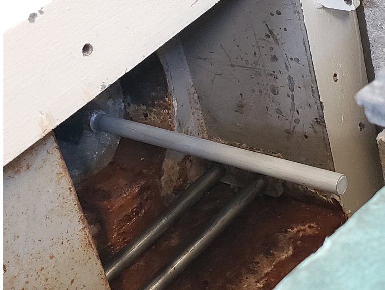
Figure 4.4: A view of the gold foil tube inserted into the NEBP collimator.
