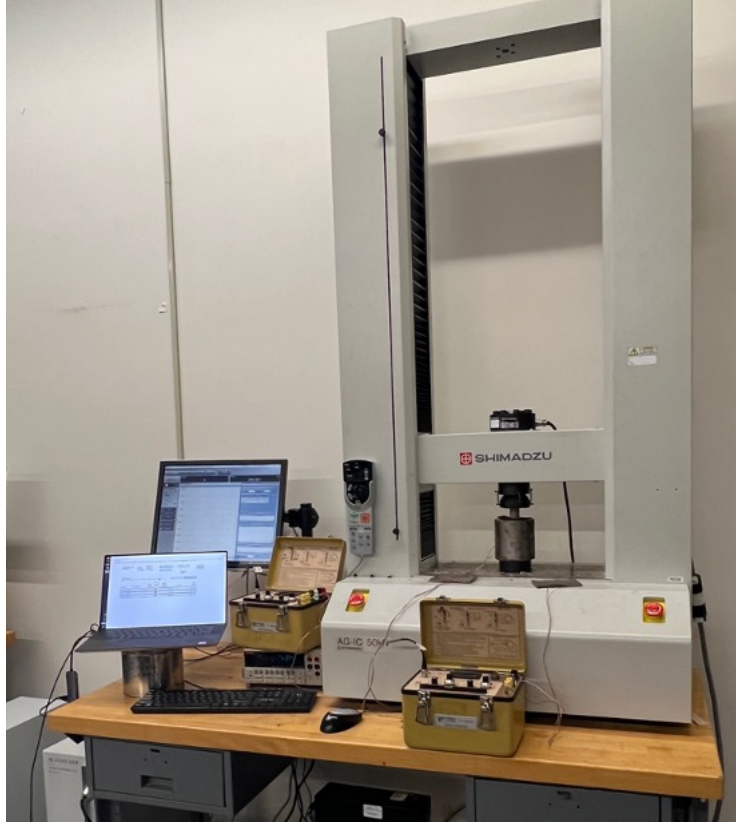
Figure 2.4 Experimental setup for uniaxial compression tests, including the Shimadzu AGIC loading device, P3500 strain indicator, and Keithley 2700 data acquisition system
