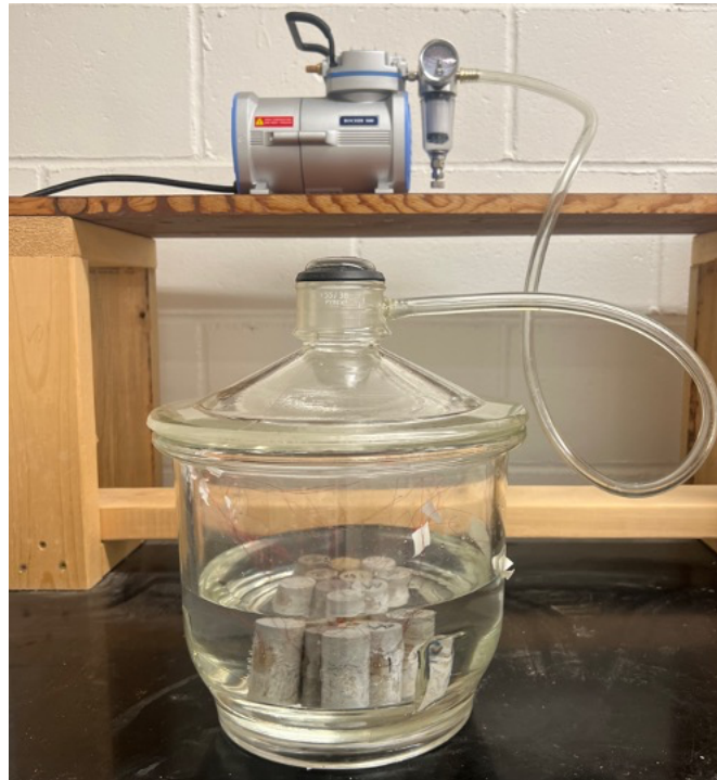
Figure 2.5 Vacuum saturation setup with glass desiccator, deionized water, connected vacuum pump, showing submerged core samples.
