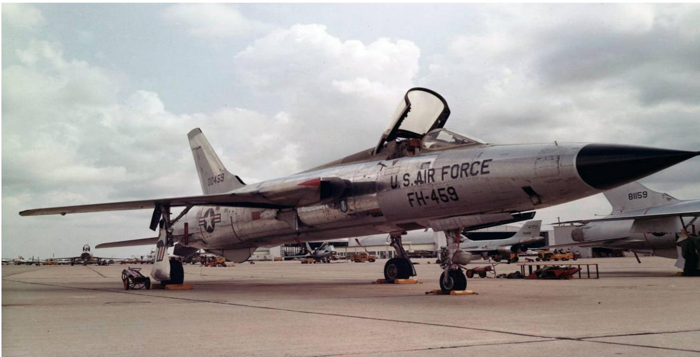
Figure B.3 F-105 in clean configuration.<sup>3</sup>
