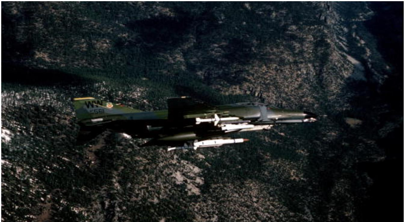
Figure B.12 F-4 *Wild Weasel* Carrying *Shrike* (outboard), *Maverick* (mid-wing), and *Standard* (inboard) on external pylons.<sup>12</sup>
