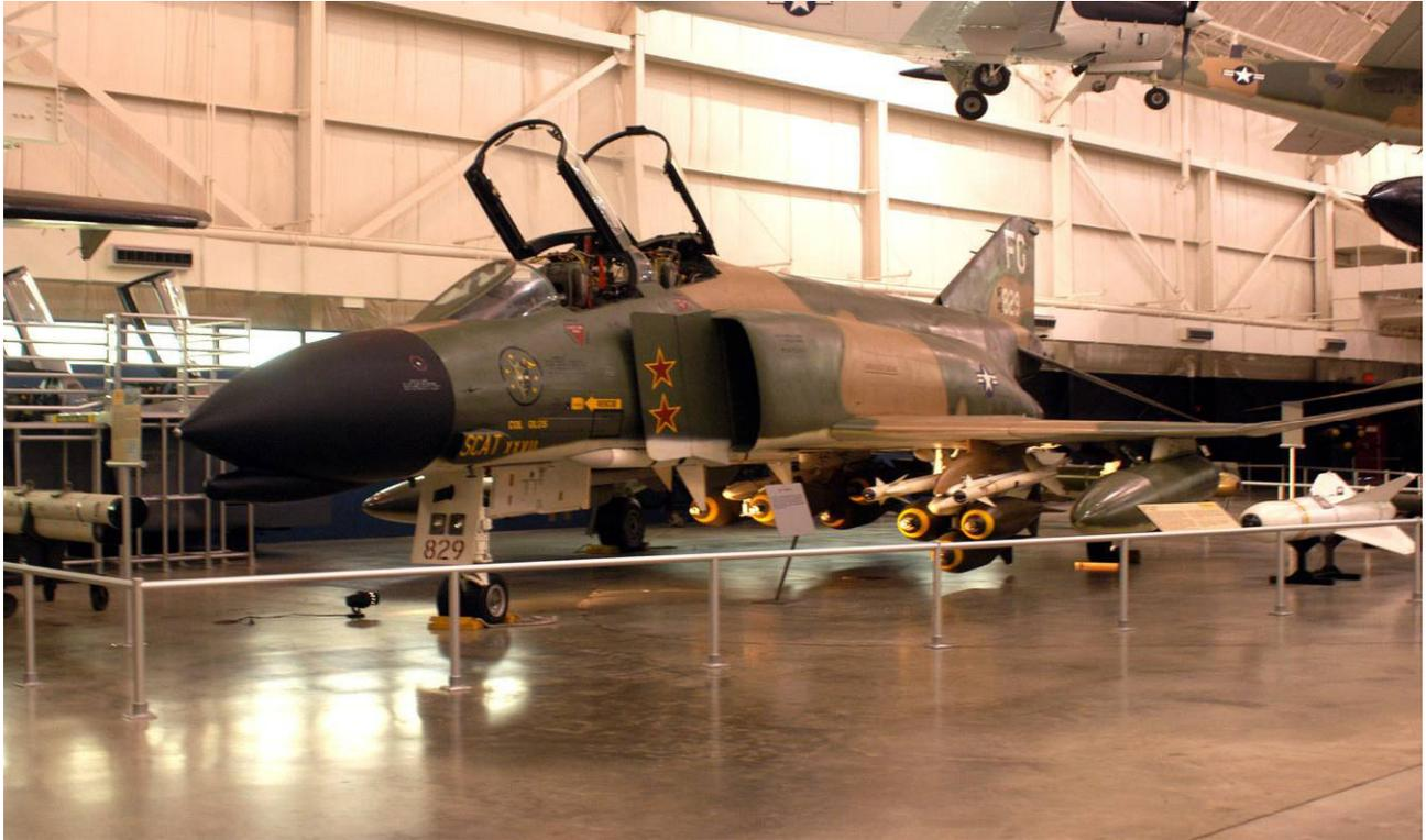
**Figure B.14 F-4C configured for multi-role mission. This was the usual configuration for *Phantoms* tasked with an air-to-ground primary mission followed by a secondary air-to-air encounter. This particular F-4C was Colonel Olds' mount during Operation Bolo.<sup>14</sup>**
