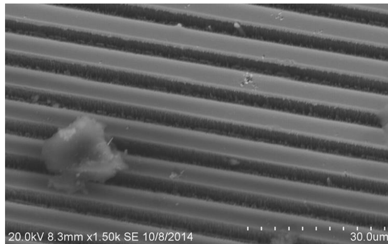
Figure 4-50: SEM image of the evaporated Ti/Au contact on an etched device. The region to the top right is the region that the material was deposited. Material was prevented from depositing on the bottom-left region by the Kapton tape.
