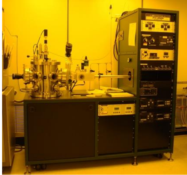
Figure 5-20: Sputtering system, used for the deposition of metals such as titanium or gold and other materials including indium tin oxide (ITO), silicon dioxide, and boron [32].
