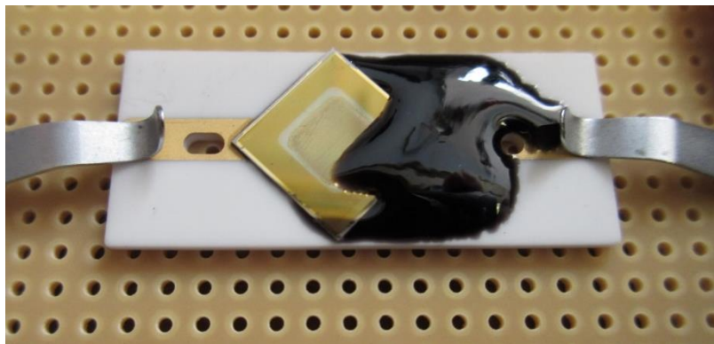
Figure 5-23: Photo of the SiC device after being mounted, wirebonded, and epoxied onto an alumina substrate for testing.
