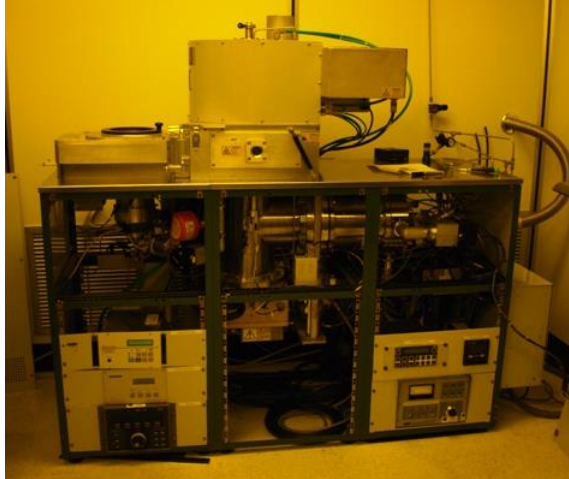
Figure 4-7: Oxford PlasmaLab 100 ICP-RIE used for etching microstructures within the SiC devices [32].
