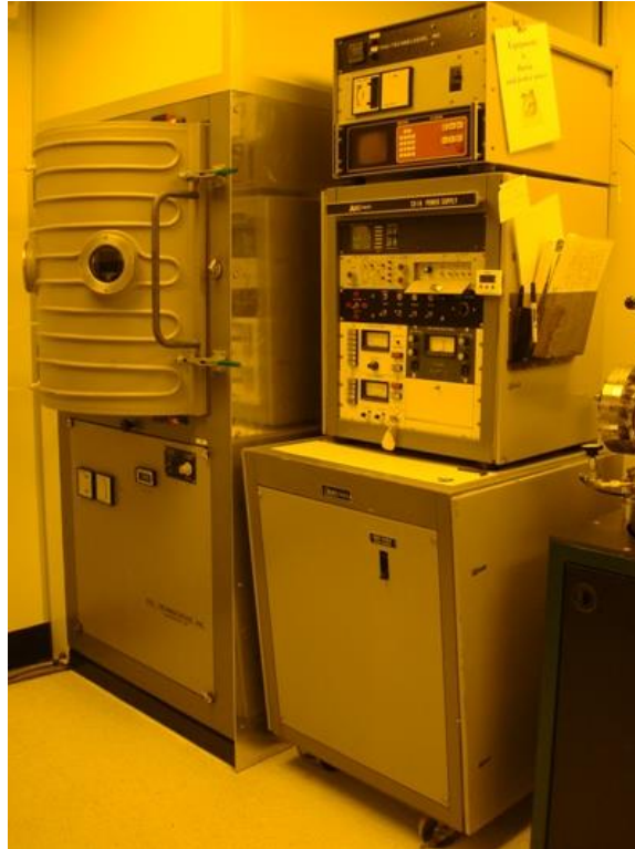
Figure 4-3: E-beam evaporator used for depositing contact and etchant mask layers onto silicon carbide wafers [32]. The system was capable of depositing several different materials sequentially such as titanium, gold, ITO, nickel, aluminum, copper, platinum, or chromium.
