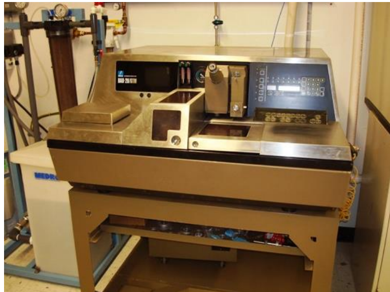
Figure 4-4: KSU S.M.A.R.T. LAB Disco DAD dicing saw. This saw was utilized for dicing the SiC wafers and was equipped with a diamond saw blade [32].
