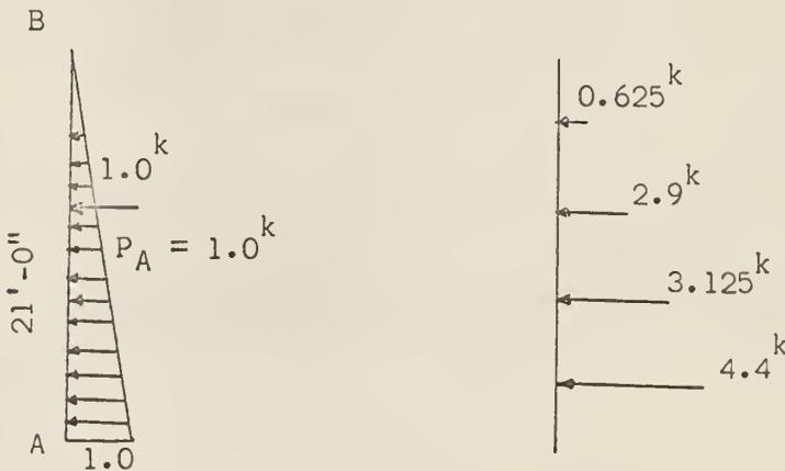
Fig. 12. Earth Pressure Diagram
