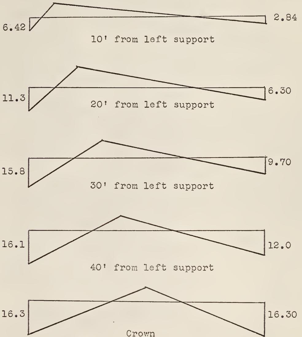
Deck Moment Diagrams for Unit Load at Each Load Point
