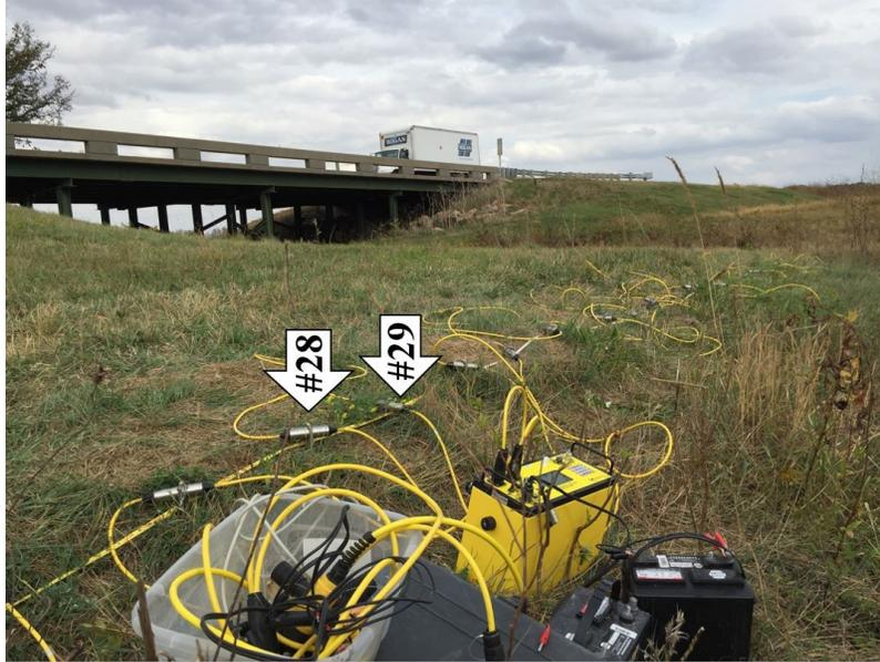
**Fig. 3.3 In situ ERT survey line including the data acquisition system.**
