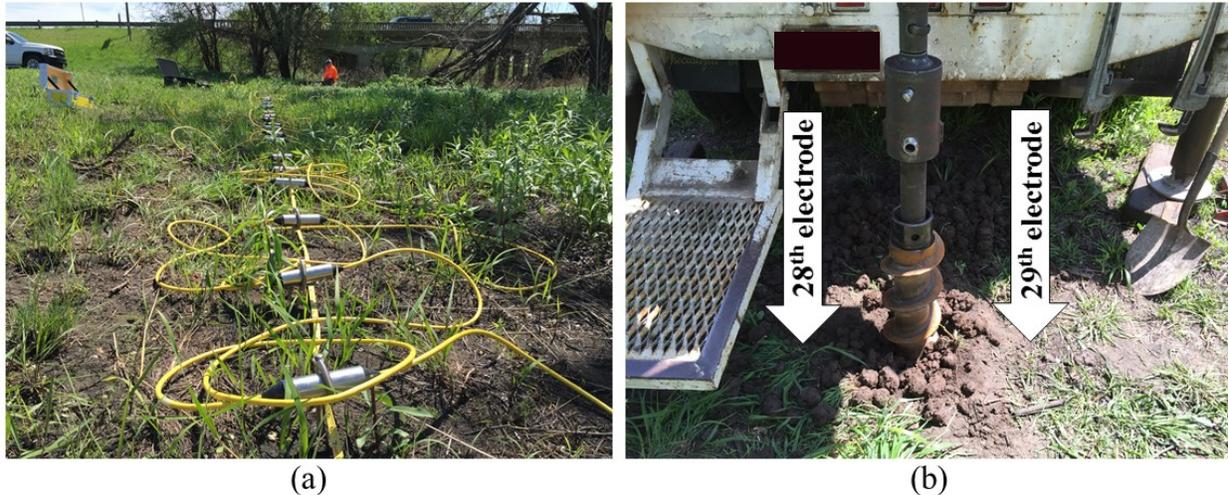
**Fig. 2.2 Experimental setup at the bridge sites: (a) ER survey line; (b) potential position of 28th and 29th electrodes around borehole**
