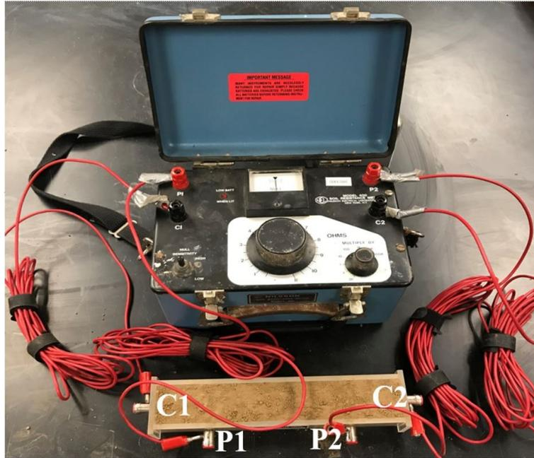
**Fig. 3.4 Resistance meter and soil box with C1, C2 current electrodes and P1, P2 voltage electrodes.**
