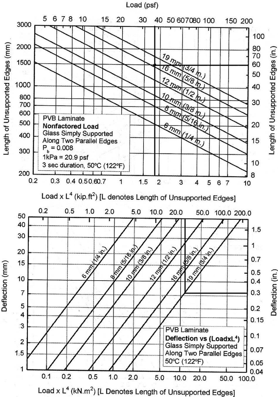
FIG. A1.41 (upper chart) Nonfactored Load Chart for Laminated Glass Simply Supported Along Two Parallel Edges
