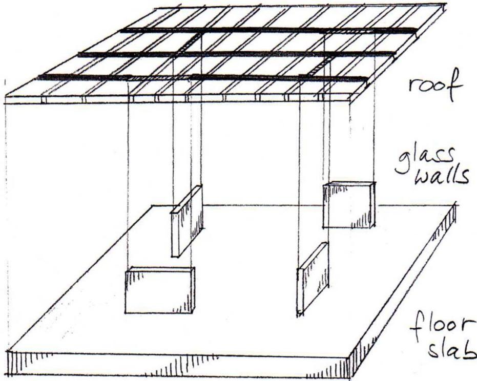
**Figure 8-1 Sketch of Structural Glass Wall and Roof Structure (Nijse 108)**
