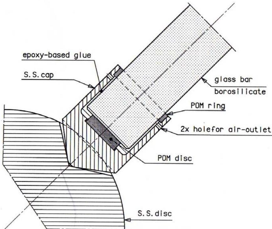
**Figure 7-2 Glass Truss Connection** (Nijse 64)
