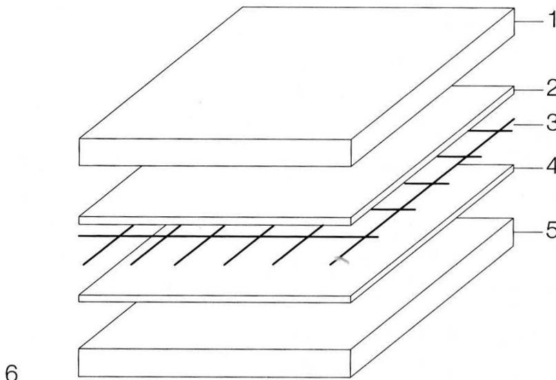
**Figure 4-3 Armored Laminated Glass Structure** (Kaltenbach 35)
