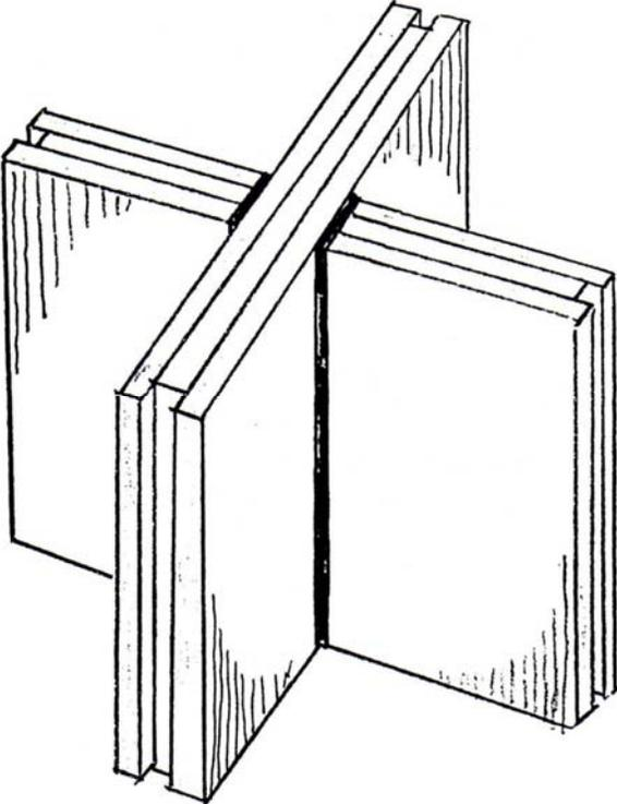
**Figure 5-4 Cross-Shaped Column** (Nijse 72)
