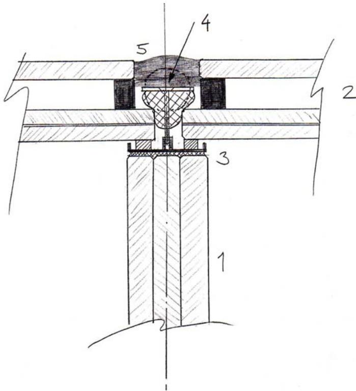
**Figure 7-3 Connection Detail for Glass Beam to Insulated Glass Panel (Nijssse 24)**
