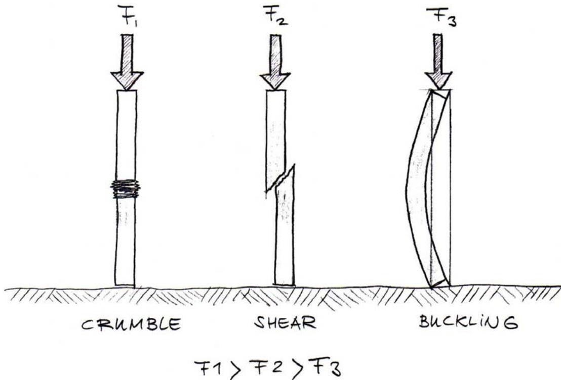
**Figure 5-2 Failure Modes of Columns** (Nijssse 60)
