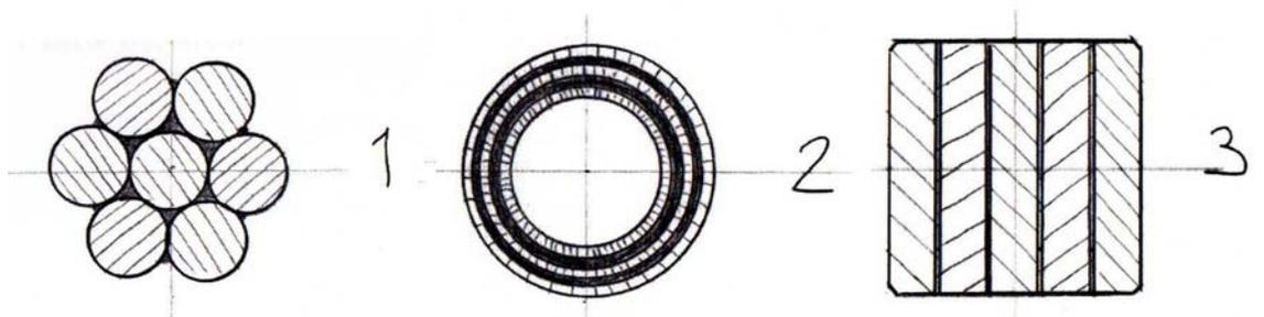
**Figure 5-3 Laminated Glass Column Configurations** (Nijssse 69)
