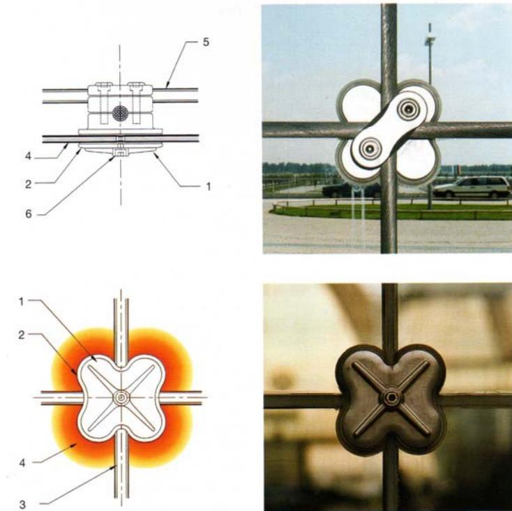
**Figure 7-5 Point-Fixing Glazing Connection (Loughran 20)**
