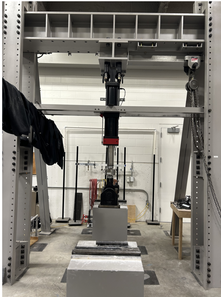
Figure 20: Test Frame and Concrete Support
