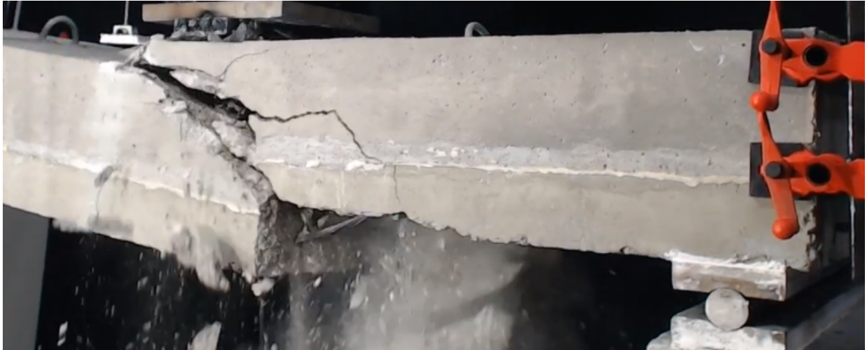
Figure 40: 6-foot 7-Wire Strand Failure
