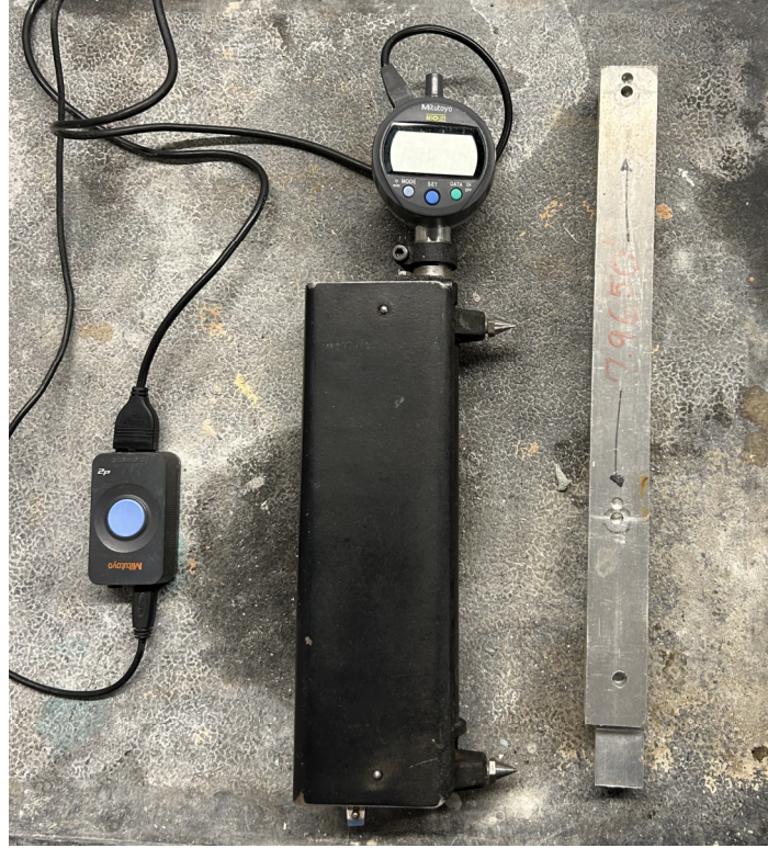
Figure 13: Whittemore Strain Gage and Zero Block
