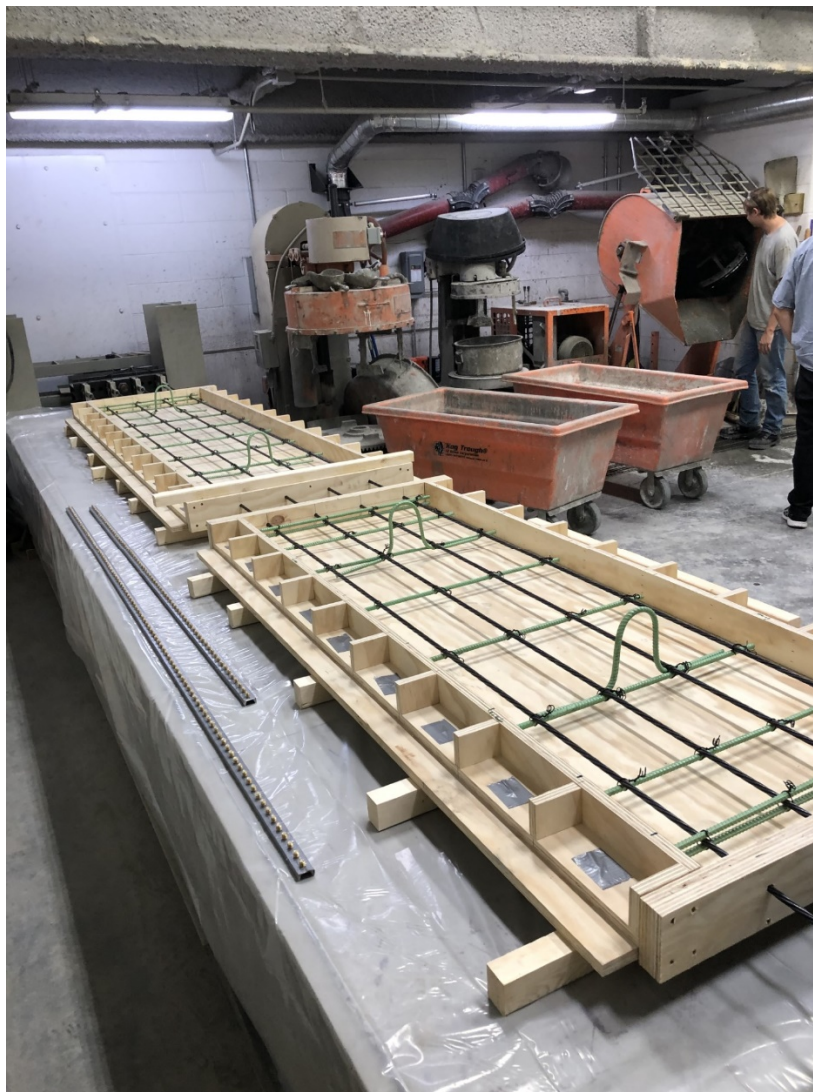
Figure 10: Tensioned Tendons and Panel Forms
