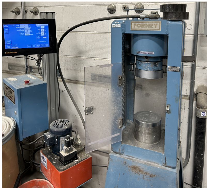
Figure 15: Forney 250 Series Frame with VFD Controls
