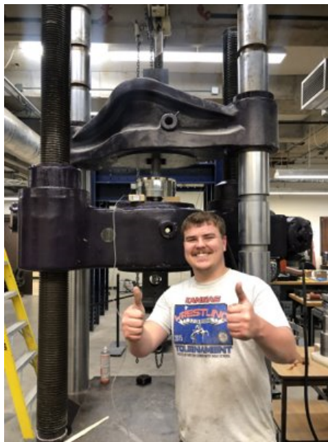
Figure 7: Calibration of "Pancake" Load Cell
