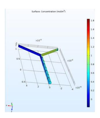
Diameter = 500 microns Channel Height = 15 mm Chip Dimensions = 3.3 x 1.8 cm
