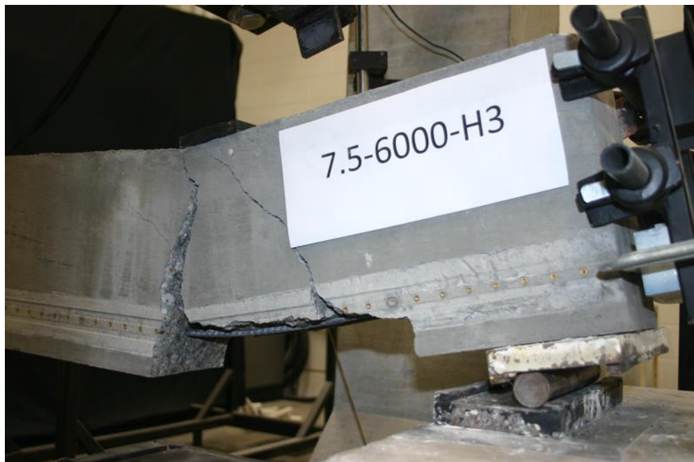
Figure 4.23: Development of Flexural-Shear Crack Leading to Spalling and Bond Failure of Specimen 7.5-6000-H3.
