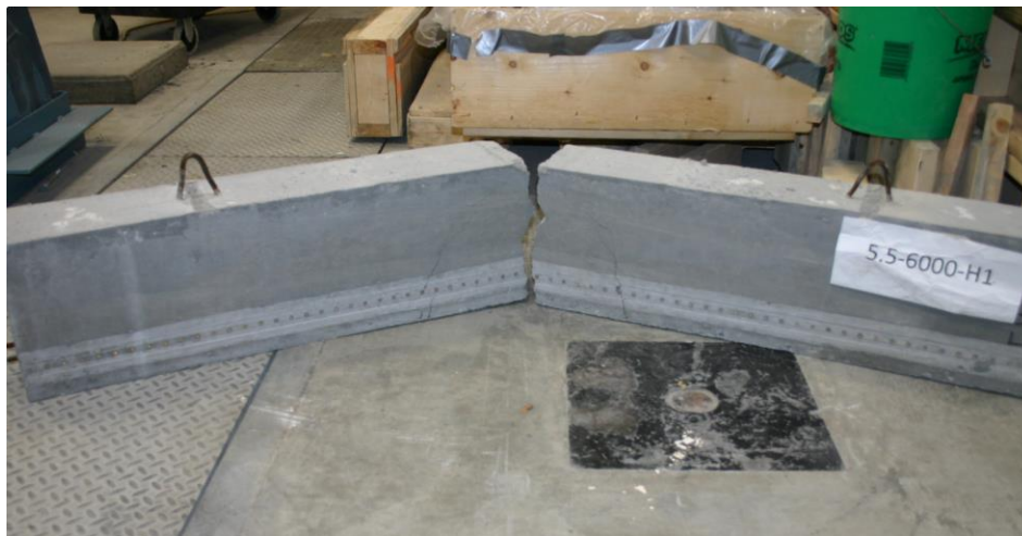
Figure D.35: Broken Beam Failing Through Strand Rupture.
