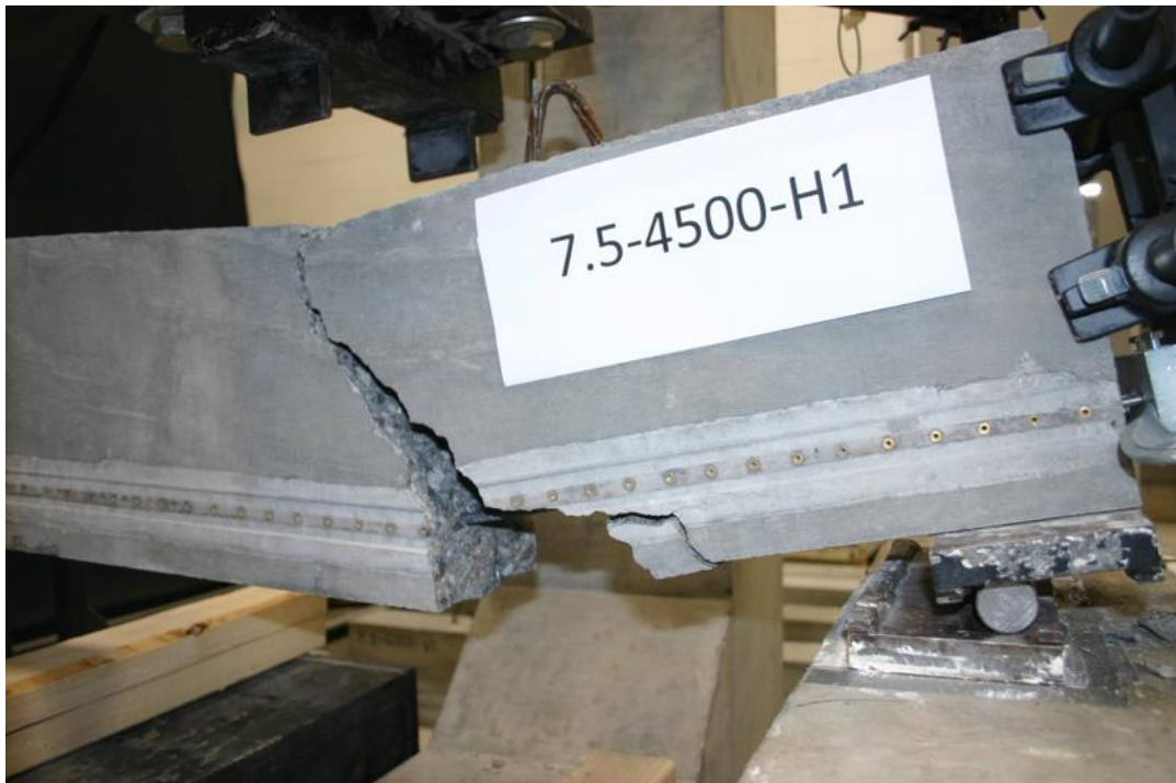
Figure 4.21: Flexure-Shear Crack During Flexural Testing Leading to Spalling of Concrete and Bond Failure.
