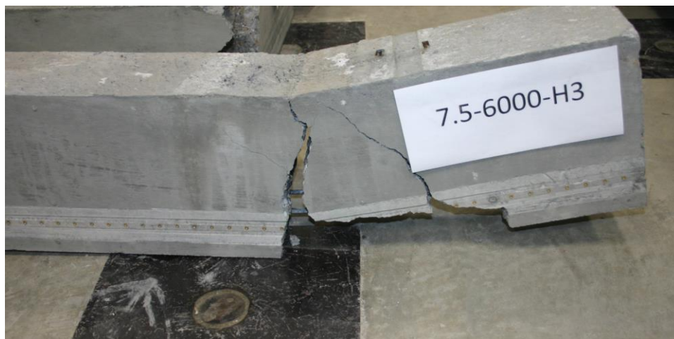
Figure D.45: Broken Beam Failing Through Loss of Bond.
