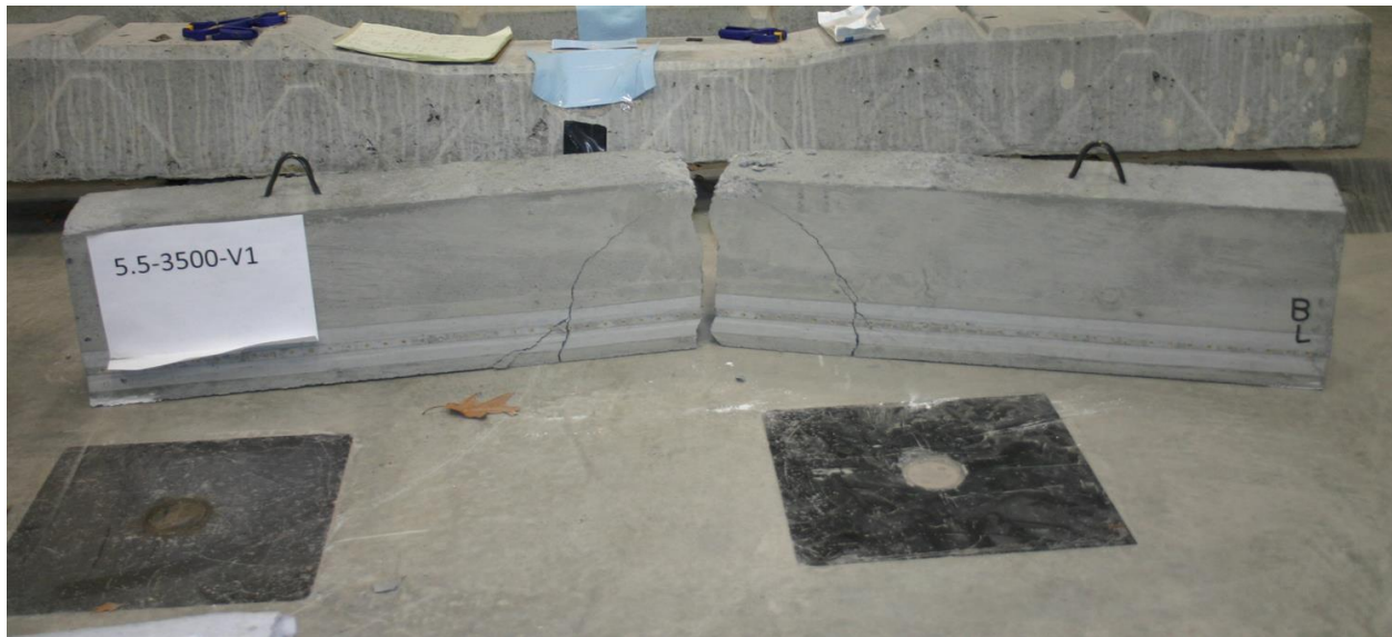
Figure D.11: Broken Beam Failing Through Strand Rupture.
