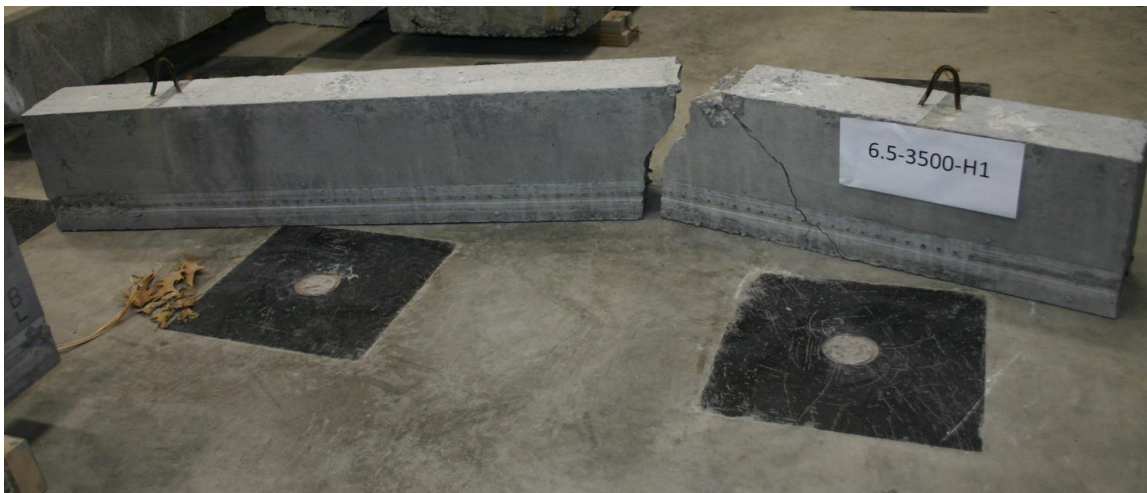
Figure D.3: Broken Beam Failing Through Strand Rupture.
