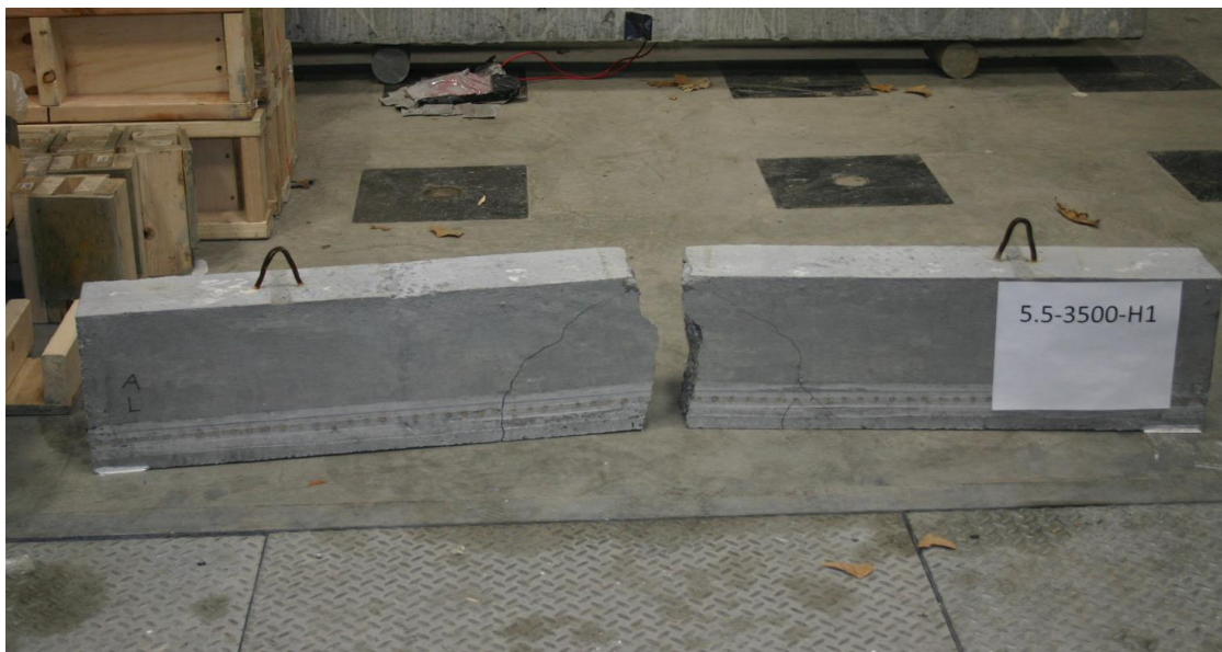
Figure D.1: Broken Beam Failing Through Strand Rupture.
