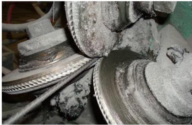
Figure 3.4: Indentation Rollers During Manufacturing of Indented Prestressing Wire (Beck et al., 2019).
