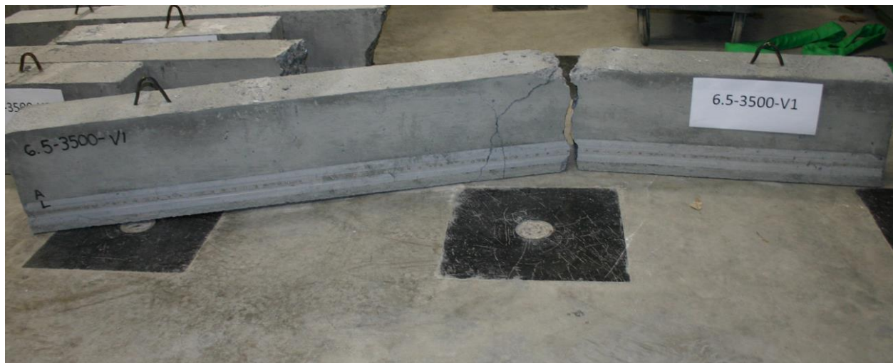
Figure D.13: Broken Beam Failing Through Strand Rupture.
