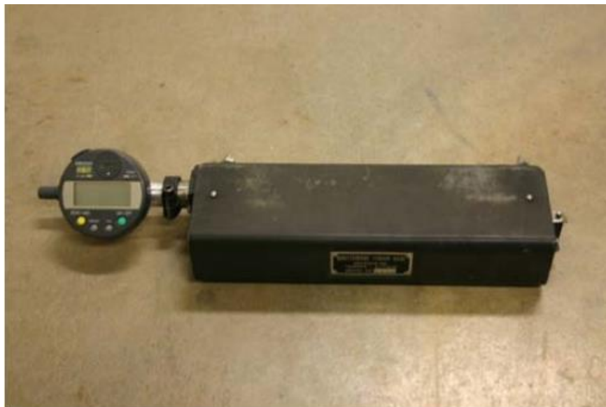
Figure 3.18: Whittemore Gauge Used in Surface Displacement Data Collection.
