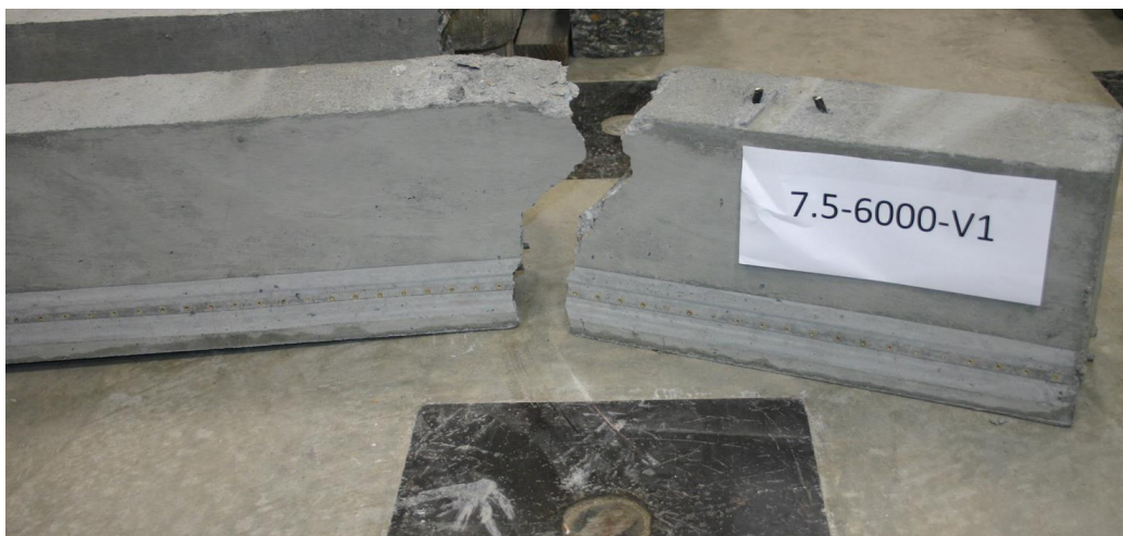
Figure D.51: Broken Beam Failing Through Strand Rupture.
