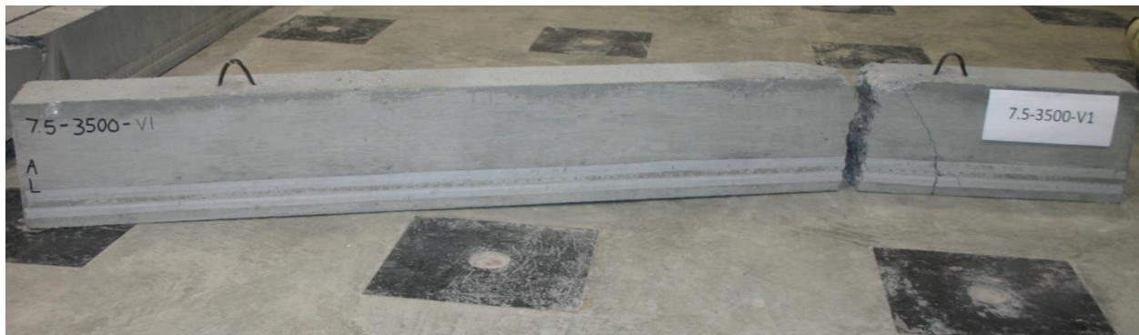
Figure D.15: Broken Beam Failing Through Strand Rupture.
