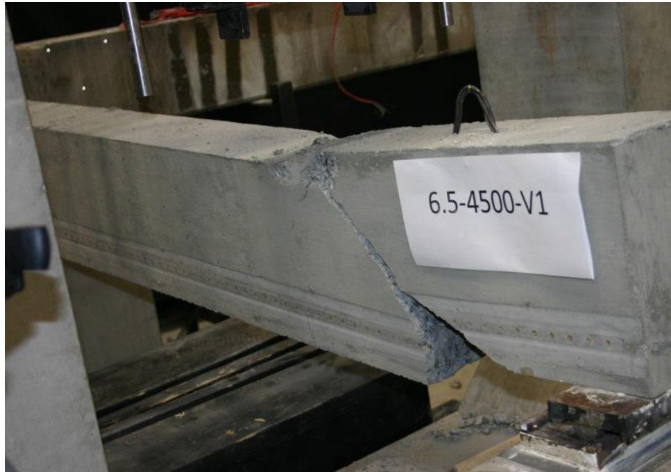
Figure 4.13: Development of Flexural-Shear Crack During Testing of Specimen 6.5-4500-V1.
