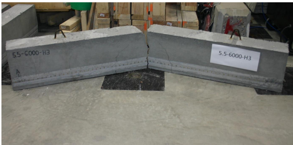
Figure D.41: Broken Beam Failing Through Strand Rupture.
