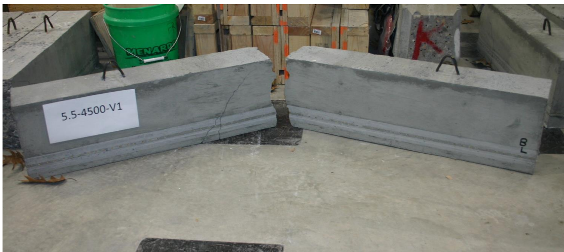
Figure D.29: Broken Beam Failing Through Strand Rupture.
