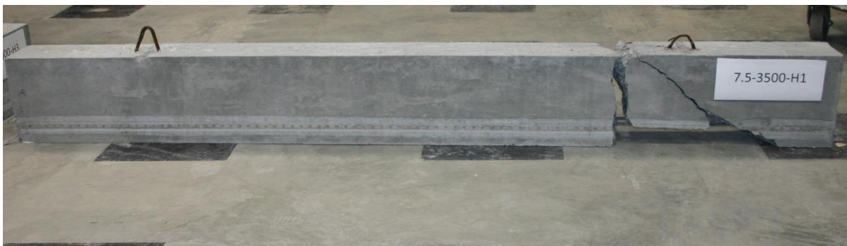
Figure D.5: Broken Beam Failing Through Loss of Bond.
