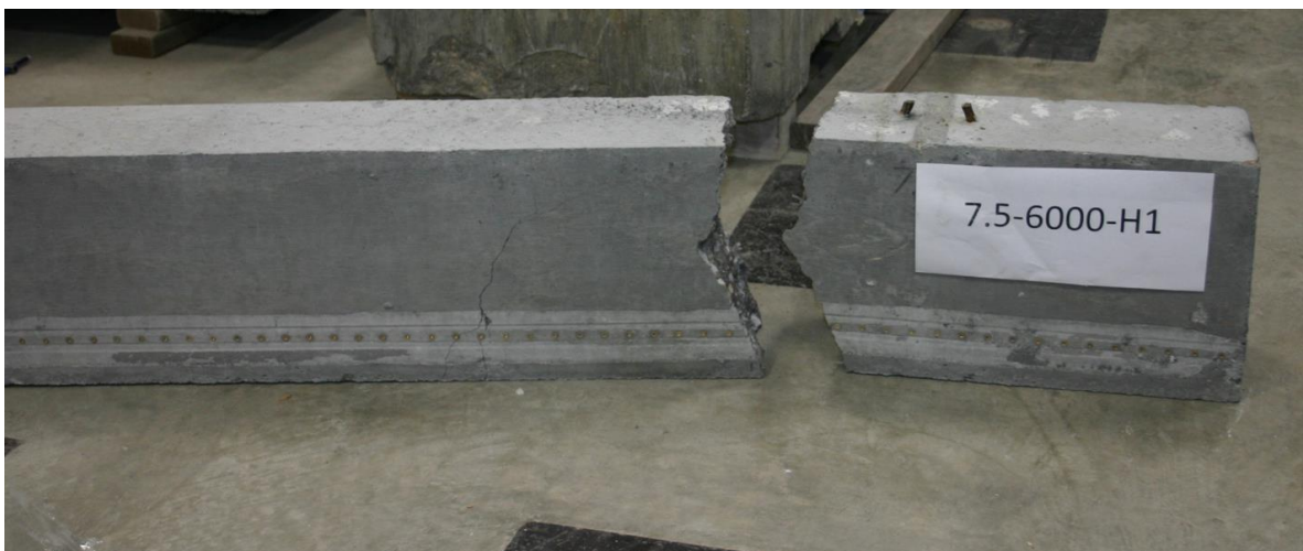
Figure D.39: Broken Beam Failing Through Strand Rupture.
