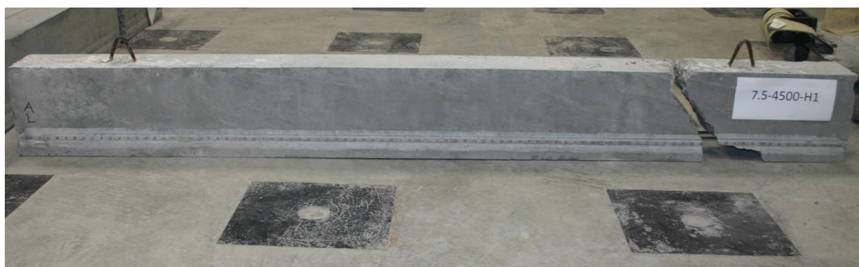
Figure D.21: Broken Beam Failing Through Loss of Bond.
