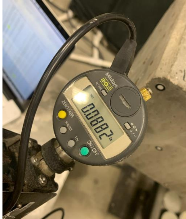
Figure 3.19: Mitutoyo Absolute Digimatic Indicator Used in Surface Displacement Data Collection.
