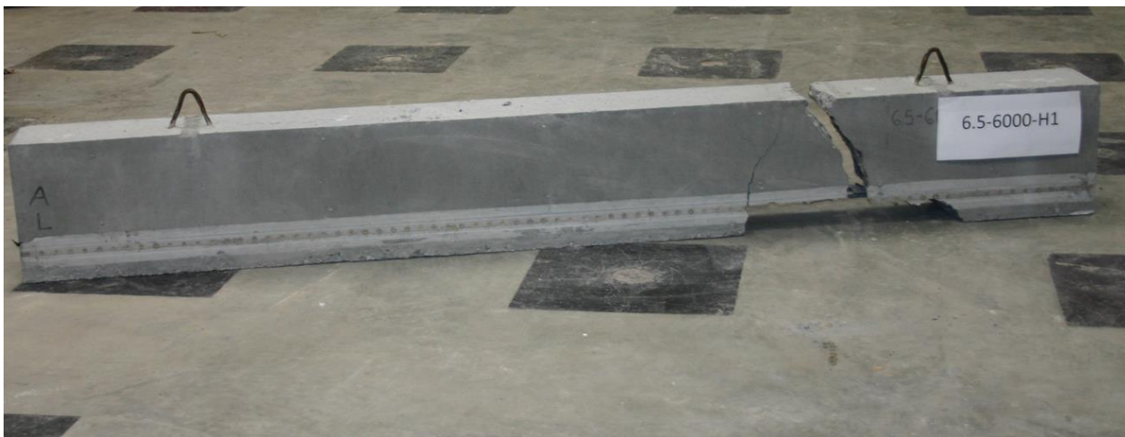
Figure D.37: Broken Beam Failing Through Loss of Bond.
