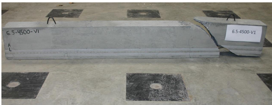
Figure D.31: Broken Beam Failing Through Loss of Bond.
