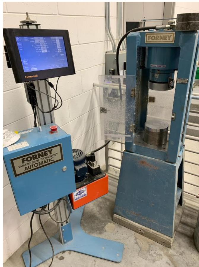
Figure 3.13: Forney Hydraulic Press Used to Perform Cylinder Tests.
