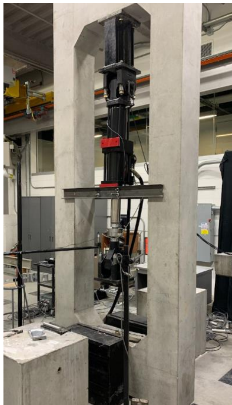
Figure 3.20: Prestressed Concrete Loading Frame Used for Flexural Testing of Specimens.
