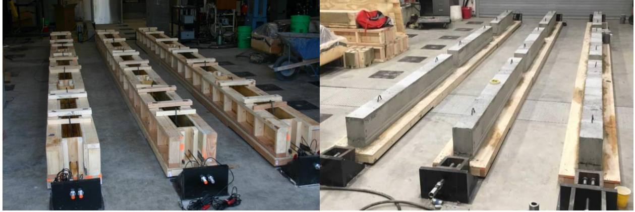
Figure 3.10: Formwork for Specimen Fabrication and After Curing.
