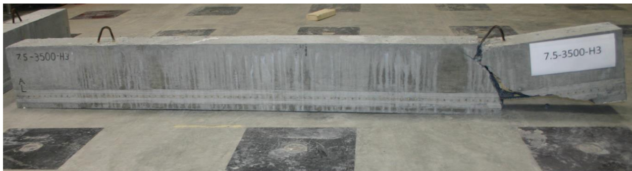
Figure D.10: Broken Beam Failing Through Loss of Bond.
