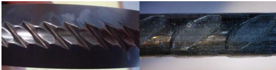
Figure 3.5: Wire Roller and Prestressing Wire After the Indentation Process (Beck et al., 2019).
