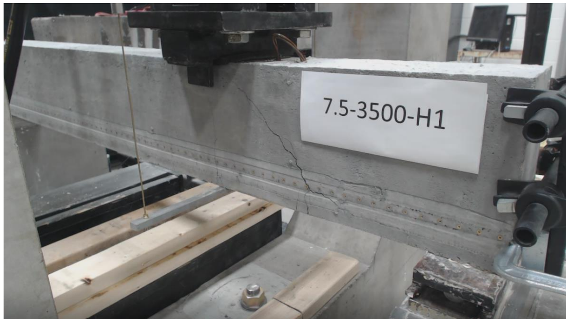
Figure 4.17: Initial Development of Flexural-Shear Crack During Flexural Testing of Specimen 7.5-3500-H1.
