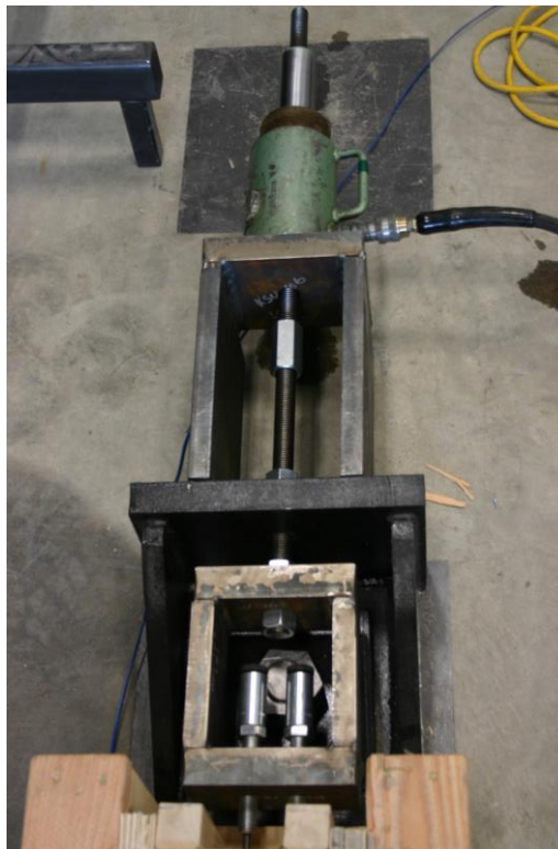
Figure 3.15: Prestressing Configuration at the Jacking End, or “Live End” of the Prestressing Bed.
