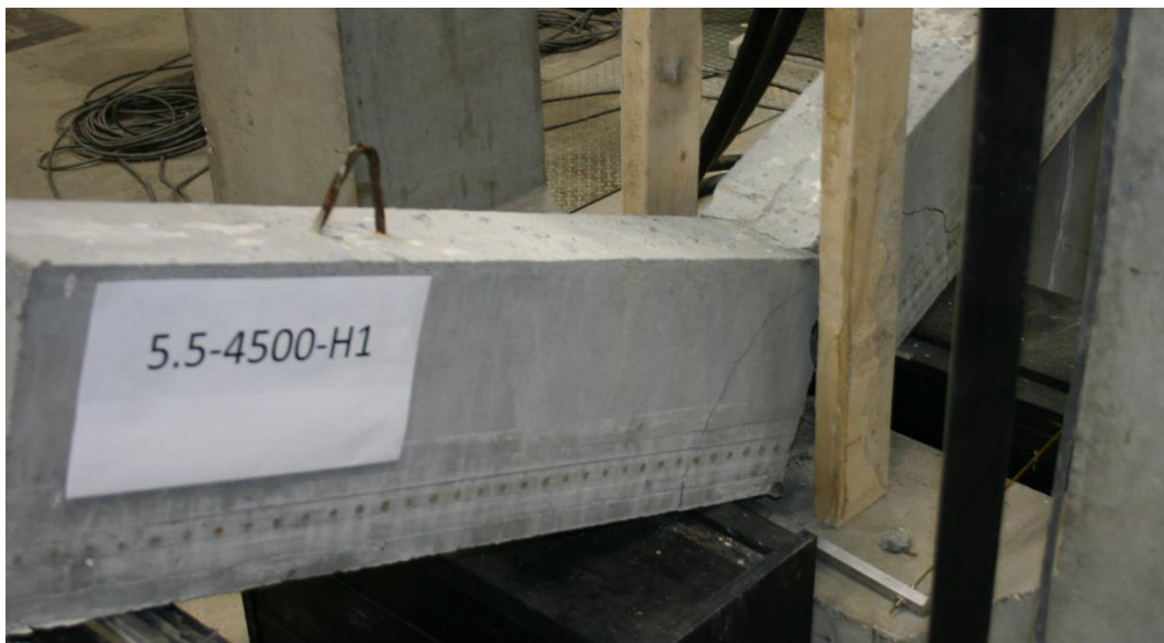
Figure D.17: Broken Beam Failing Through Strand Rupture.
