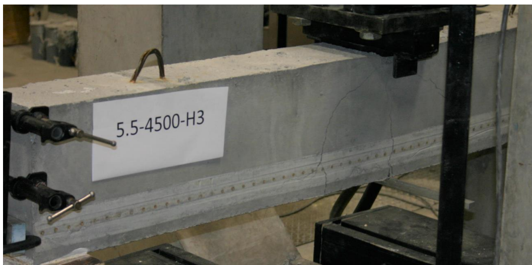
Figure D.23: Broken Beam Failing Through Strand Rupture.
