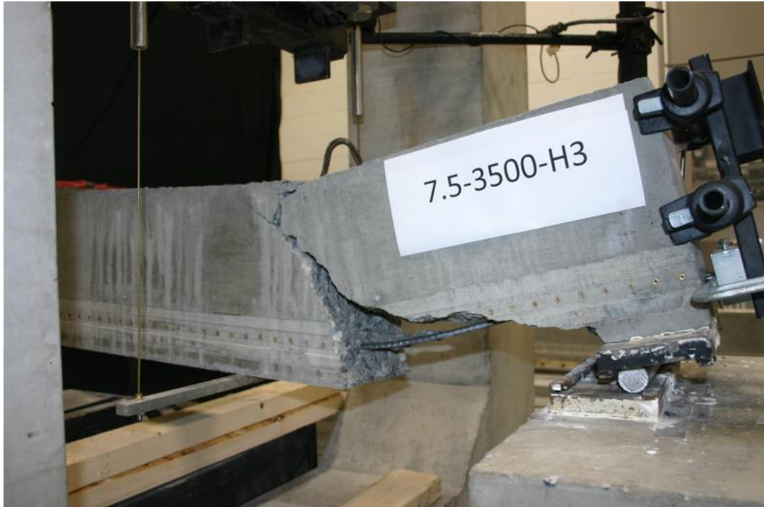
Figure 4.19: Shear Crack During Flexural Testing Leading to Spalling of Concrete and Bond Failure.
