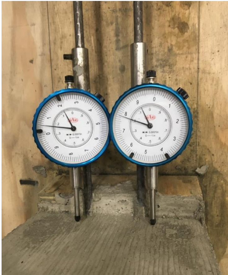
Figure 3.17: Dial Gauges Used to Measure Wire Slip During the Release of Prestress Forces.
