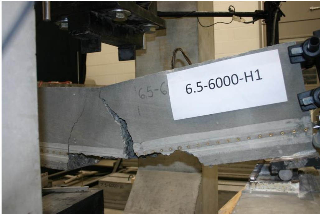
Figure 4.15: Spalling of Concrete During Flexural Testing of Specimen 6.5-6000-H1.
