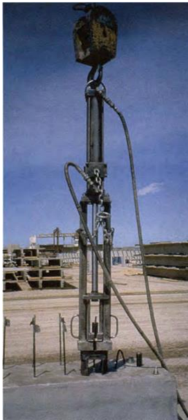
Figure 2.2: Example of Moustafa's Large Block Pull-out Test (Logan, 1997, p. 62).
