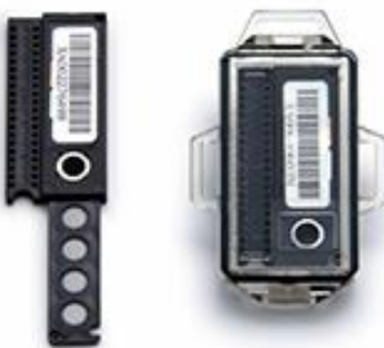
Figure 2.2. Landauer OSL-N albedo dosimeter. The ABS element casing and PET badge holder are identical to that commonly used with the Panasonic UD-802 [37].
