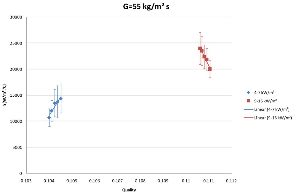
**Figure 6-35 R-134a P/D 1.5 effect of quality at 55 kg/m<sup>2</sup>.s**
