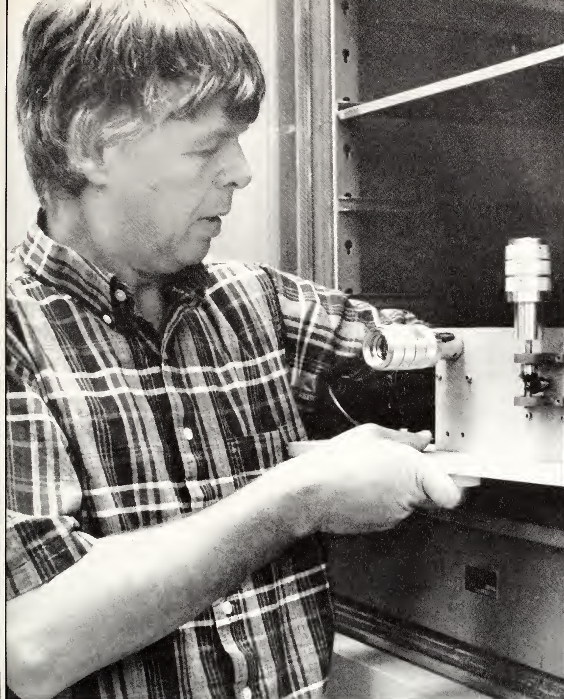
Brian Spooner, professor of biology and director of the NASA Center for Gravitational Biology, places a tissue sample into a clinostat. The clinostat simulated changes in gravity but was unable to create zero gravity. (Photo by J. Kyle Wyatt)
