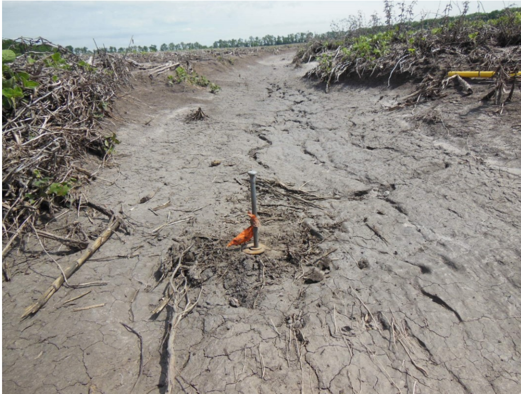
Figure 4.34 Erosion nail exposed 17 cm after 2015 spring rains
