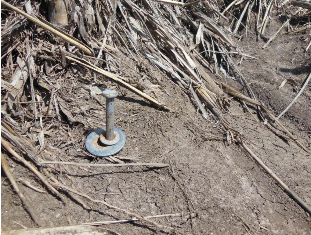
Figure 3.6 Nail and washer in gully bed, McPherson (Wedel) field, indicating erosion. Photo by author.
