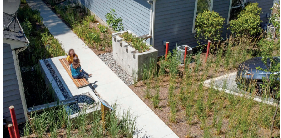
Fig 5.25: Rain gardens can be integrated within a residential landscape and can connect with gutters and help manage stormwater more holistically.
