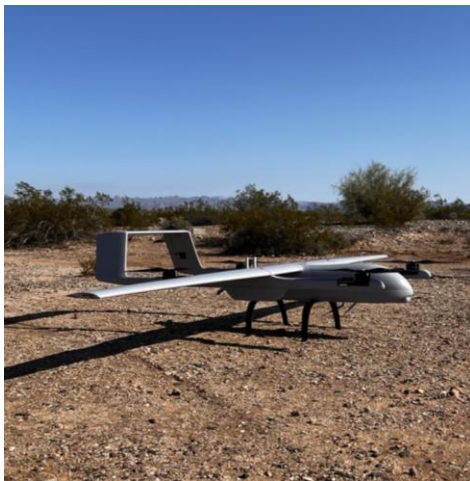
Figure 4. Hybrid VTOL UAS
