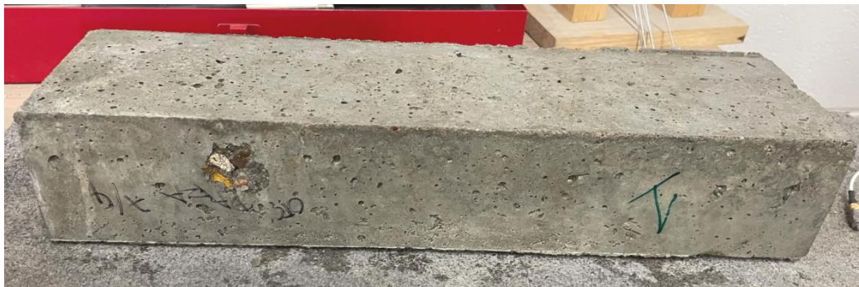
Figure 12 TYPE 1L beam 1 showing some damage to the surface
