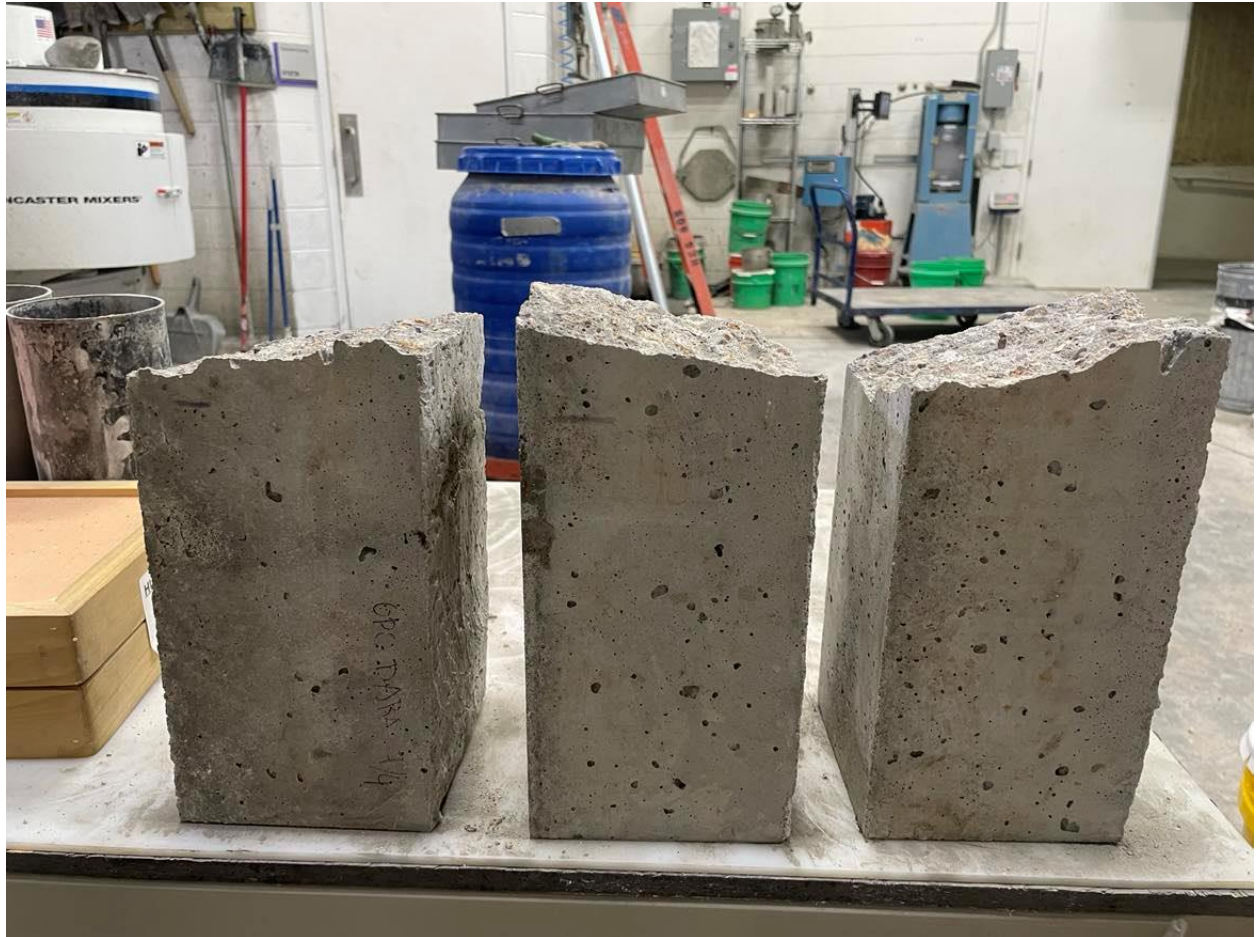
Figure B.1 Flexural Strength beams breaking within the middle 1/3 rd
