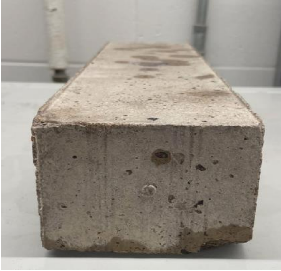
Figure 13 LC 3 beam showing small damage at the corner of the beam
