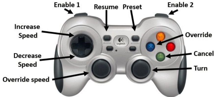
Figure 3.7: Logitech controller for Husky showing cruise control functionality.
