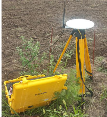
Figure 3.4: Ag542 base station mounted on tripod.
