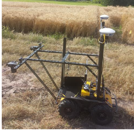
Figure 3.3: Husky mobile robot equipped with two cameras.
