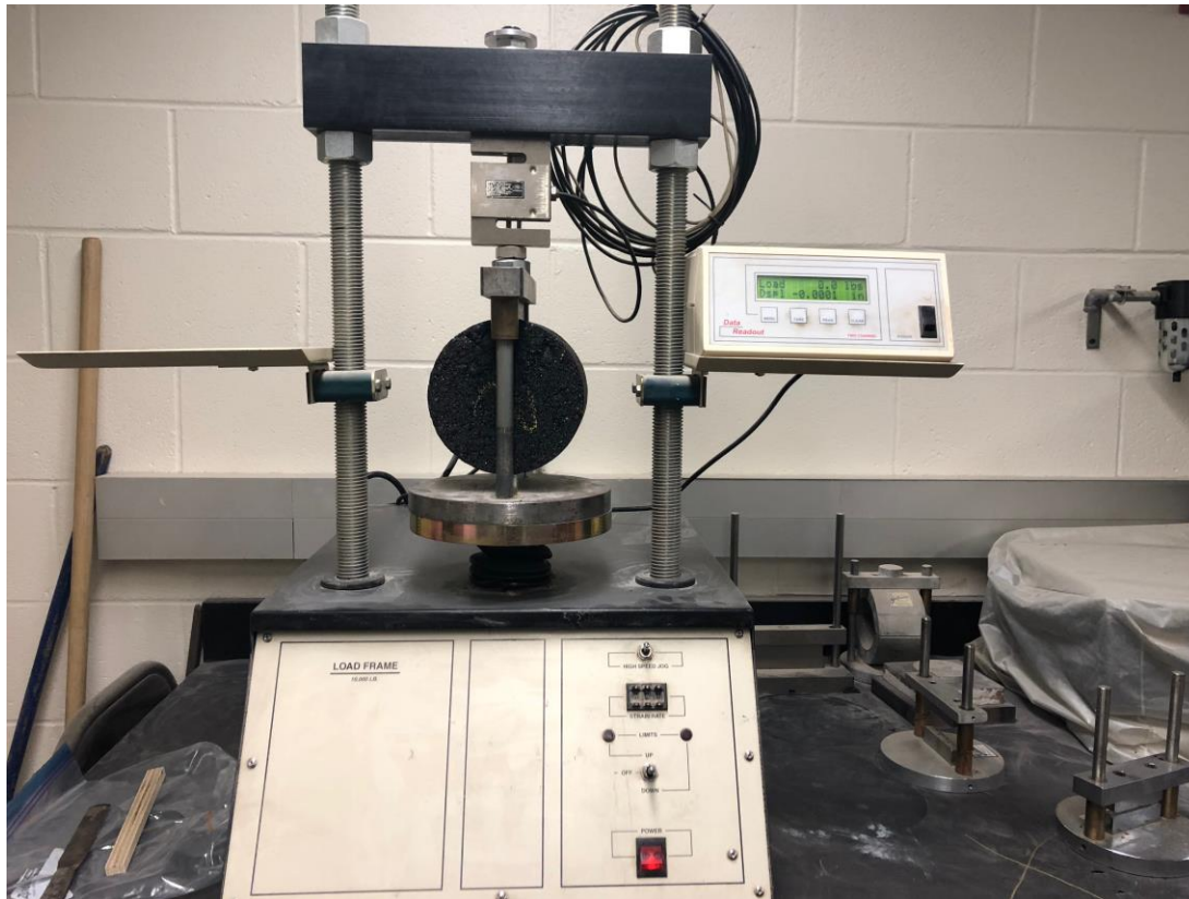
Figure 2.6. Indirect Tensile Strength Test Setup
