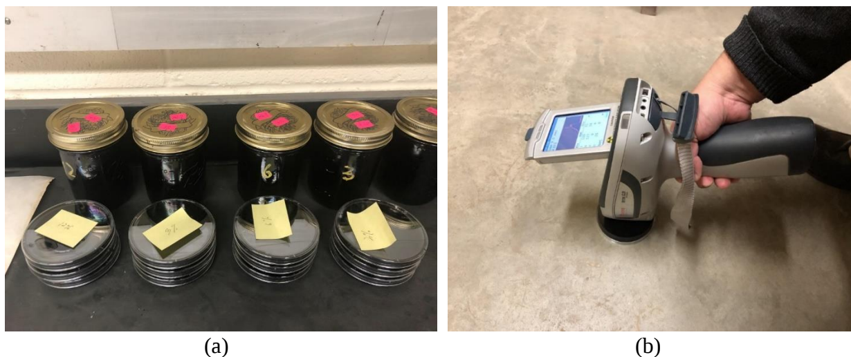
Figure 4.1. (a) Test Samples with Different REOB Content and (b) XRF Device
