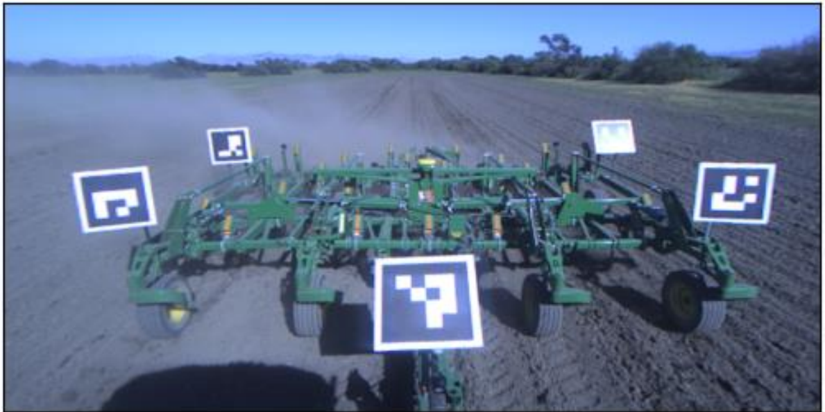
Figure 1.1 Example of ArUco markers on a 2430 CP implement
