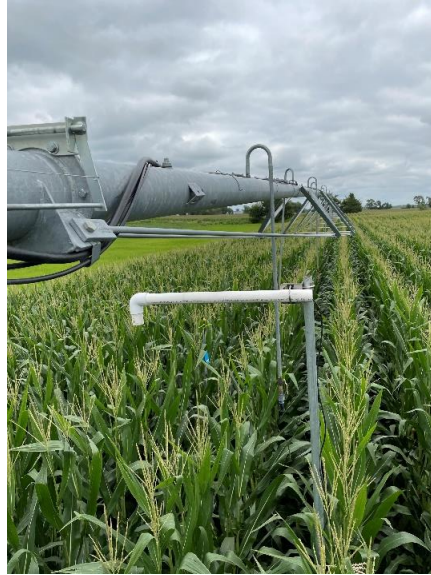
Figure 3.4. Infrared radiometer installed over corn canopy in the field
