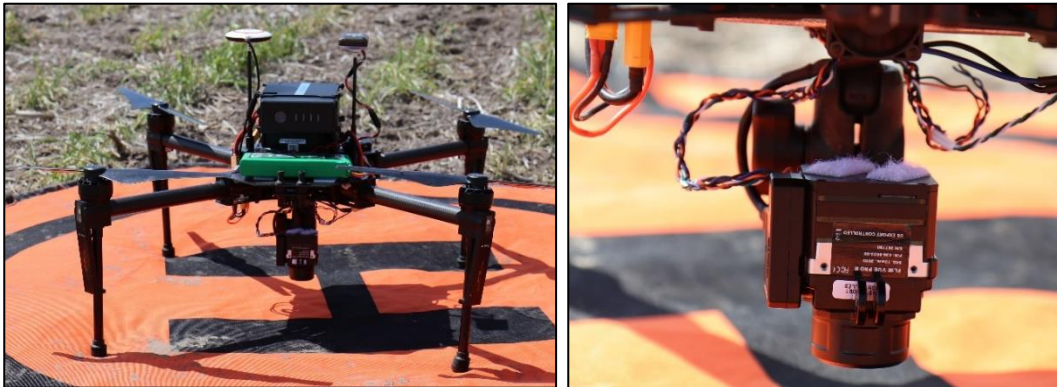
Figure 2.1. Quadcopter Matrice 100 used with the FLIR Vue pro Thermal Infrared Sensor
