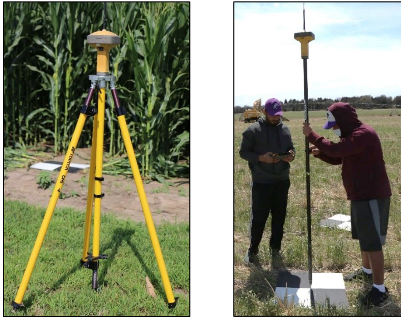
Figure 2.2. Topcon Gr-5 base station with a rover unit, for collection of RTK corrected GCPs coordinate
