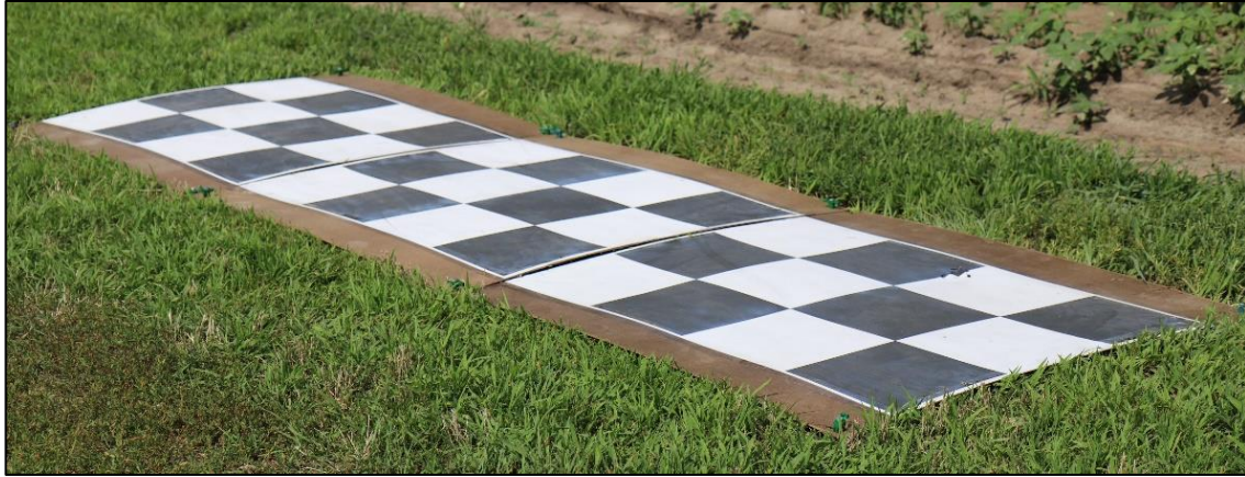
Figure 2.5. Sheet used for geometric accuracy analysis consisting black and white checkerboard boxes
