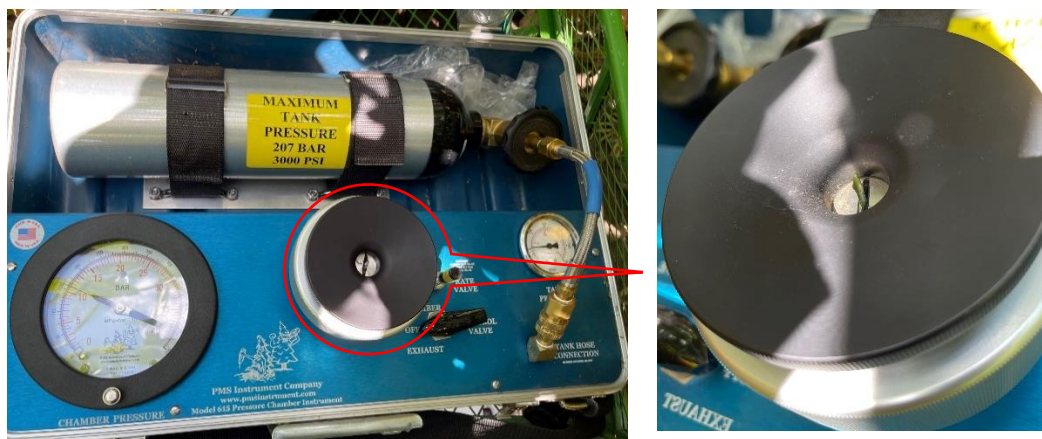
Figure 3.6 Scholander pressure chamber in the field for leaf water potential
