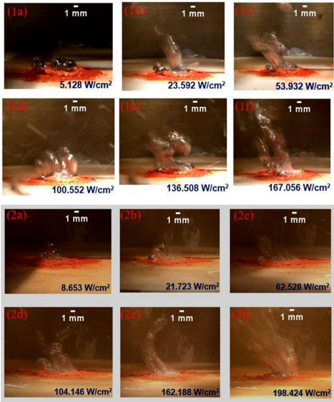
Figure 5.8 The recorded nucleate pool-boiling images for the 200 \mu\text{m} mono layer wick structure are shown in 1(a) – 1(f) at 0 psig (0 kPa) at different heat fluxes. The high-pressure boiling images at 30 psig (206.8 kPa) for the monolayer wick are shown in 2(a) – 2(f) for different heat fluxes
