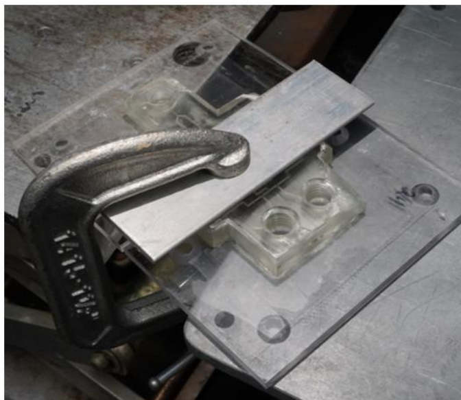
Figure 2.3. A 3D-printed microfluidic device sealed to transparency film using a combination of PVA and cyanoacrylate adhesives. Once clamped into place, as shown, water was flushed through the channels to dissolve the water-soluble PVA adhesive.
