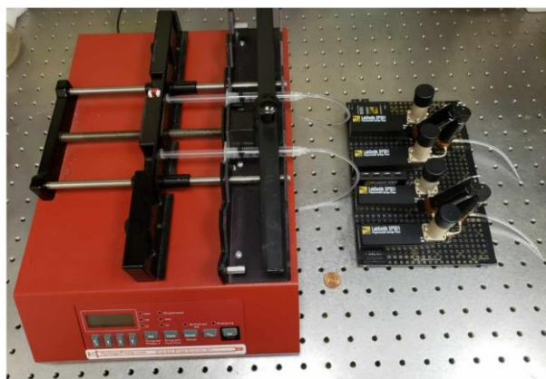
Figure 4.5. Comparison between the multi-channel syringe pump and LabSmith fluidic equipment for gradient experiments. Flat ribbon cables excluded from LabSmith equipment for clearer visual.
