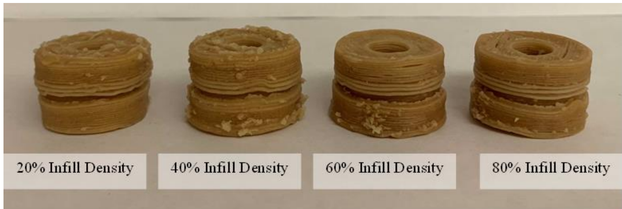
Figure 3.13. Example 3D printed samples with different infill densities using wheat-based ink.
