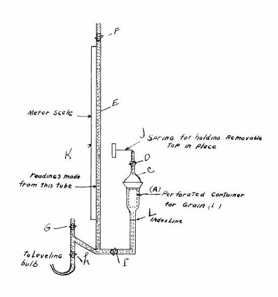
hollow glass stopper (C) drawn to a small tube at the top and closed by pet cock (D). A ground glass joint forms the union of chamber and stopper.
