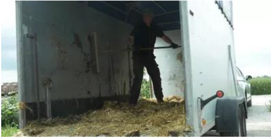
Figure 2. Manual removal of bedding and organic material from a livestock transport trailer (Karcher, 2026)
