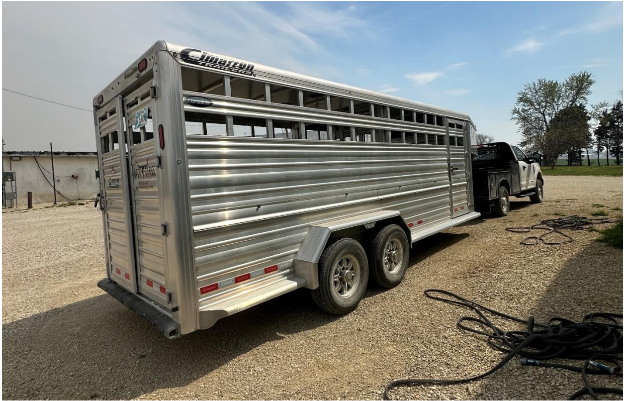
Figure 9. Cimarron livestock trailer with a tandem axle and slat-side ventilation design constructed of aluminum.
