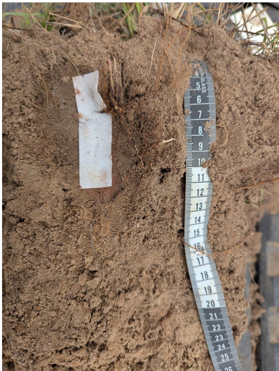
Appendix Figure G.5. West Kramer V \alpha,\alpha' -dipyridyl dye test results.
