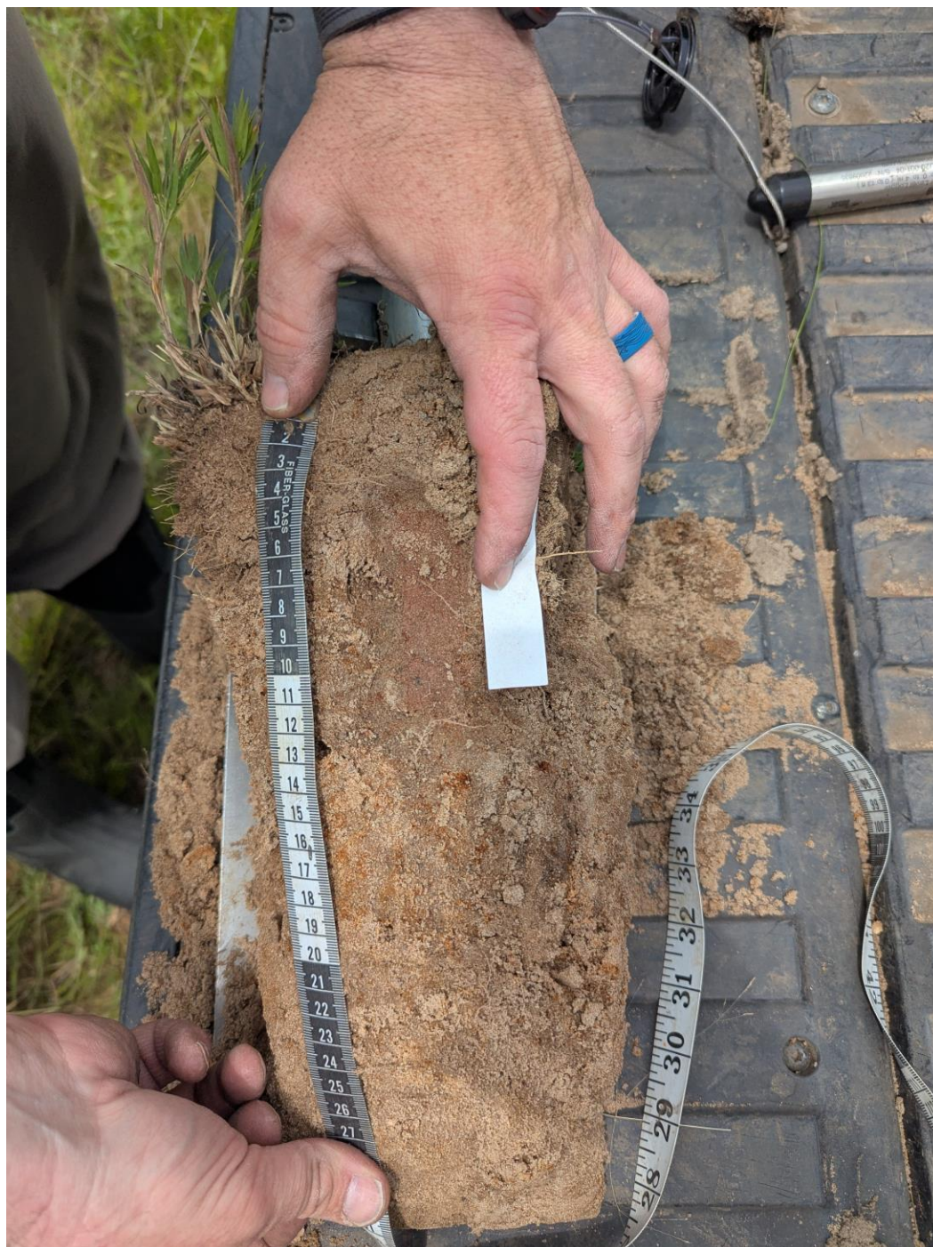
Appendix Figure G.8. Pfister D \alpha,\alpha' -dipyridyl dye test results.
