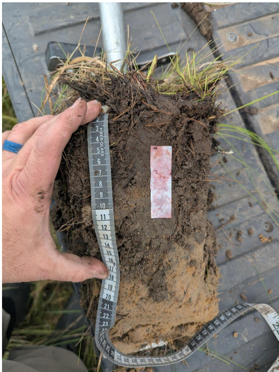
Appendix Figure G.2. East Kramer H \alpha,\alpha' -dipyridyl dye test results.
