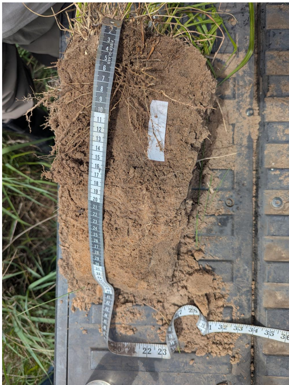
Appendix Figure G.4. West Kramer U \alpha,\alpha' -dipyridyl dye test results.
