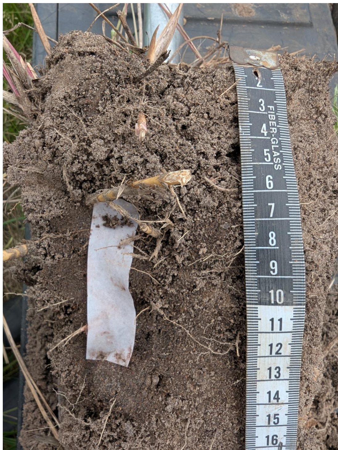
Appendix Figure G.7. Pfister B \alpha,\alpha' -dipyridyl dye test results.
