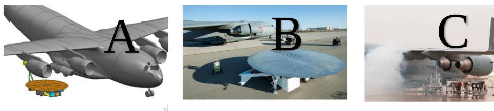
Figure 42-(a) CAD model representation of integrated C-17 and BAESS test platform (b) C-17 and BAESS test platform at EAFB prior to connection to aircraft, and (c) C-17 and platform during prior VIPR experiments
