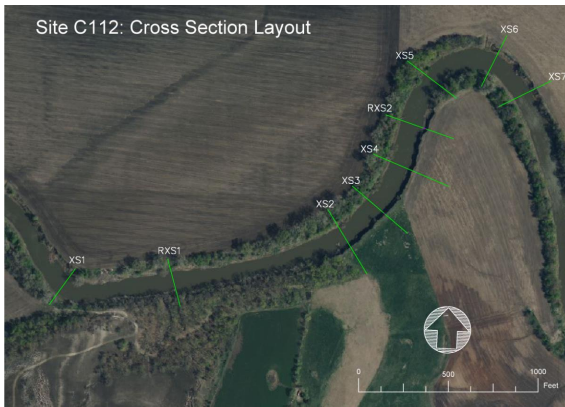
Figure 3.1 Aerial image of Site C112 with the cross section in the upstream (bottom left), middle (center), and downstream meanders (top right). XS refers to cross section, while RXS refers to riffle cross section.
