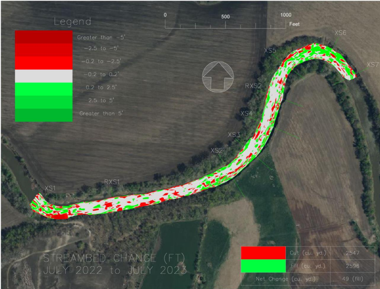
Appendix B Figure B.4 Site C112 Streambed Cut and Fill Map from 2022 to 2023
