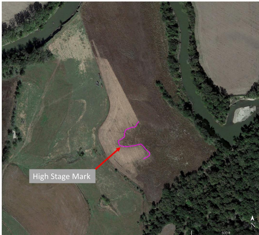
Figure 4.4 Aerial image from October 12 th , 2019, highlighting the high stage mark at Site C112.
