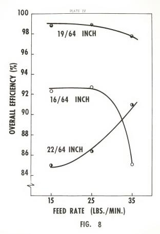
the overall efficiency of separation. As the feed rate was increased less of this material passed the screen and the overall efficiency increased. Further increases in feed rate would result in locating an optimum for this size screen.
