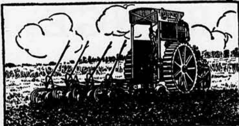
Doing a deep, even job of stubble plowing with a Hart-Parr "27" and 4 furrow self and hand lift plow.
